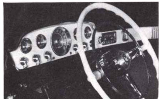
Automobile dashboards use components of "Lucite" which can pipe light around curves, and glow at the edges. "Lucite" is readily molded into complicated shapes.
