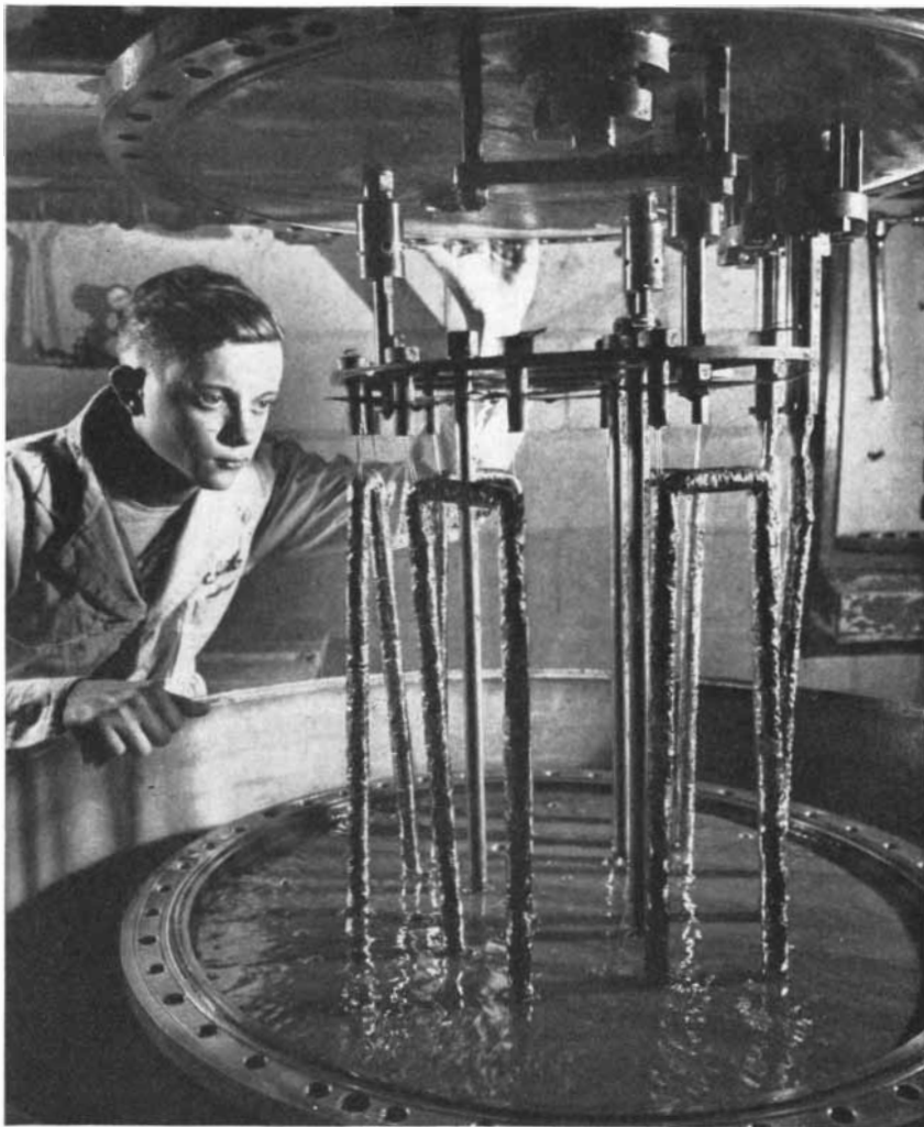
PURE ZIRCONIUM is deposited by the iodide process on the big hairpin filaments above. The base metal and iodine are heated in a vacuum, in which the filaments are suspended white hot. As the iodide vapor strikes the filaments, it decomposes, depositing the pure metal.
