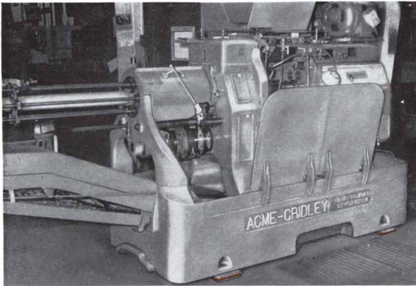
Acme-Gridley \frac{3}{16} " automatic screw machine in REPUBLIC AVIATION CORP. plant, Farmingdale, Long Island . . . showing UNISORB mounting pads under machine base. No costly floor drilling to install this machine.
