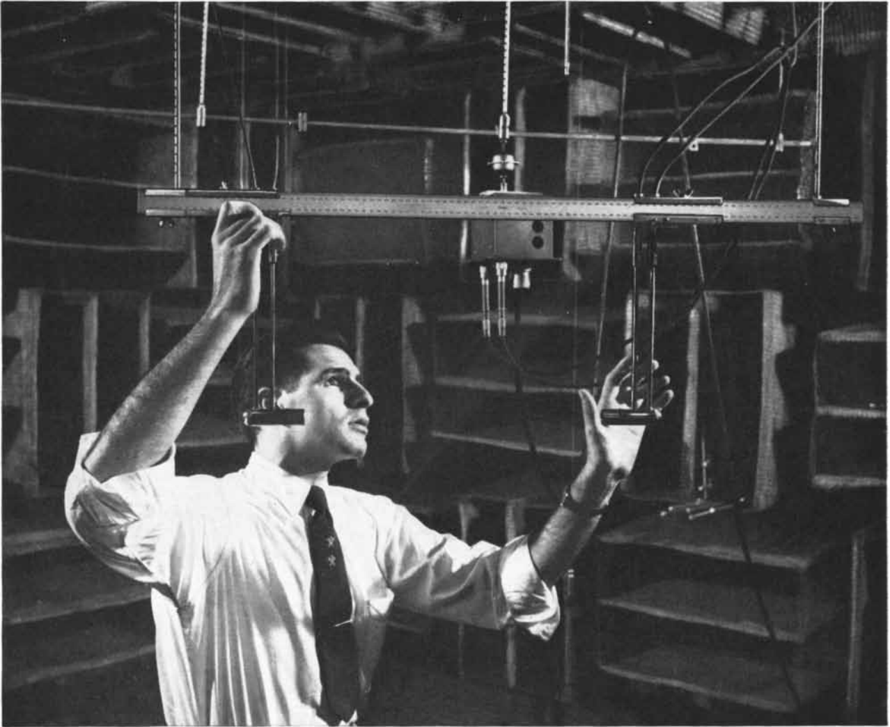
In a quiet room at Bell Laboratories an engineer scales off the distance between two condenser microphones during a calibrating test. Able to measure air pressure variations of a few billionths of an atmosphere, such microphones play a crucial role in the scientific study of telephone instruments.
