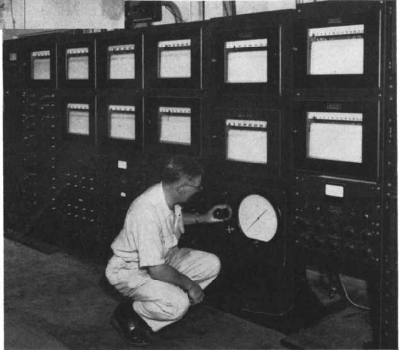
INSTRUMENTATION FOR ROCKET PERFORMANCE STUDIES utilizes this panel of Honeywell instruments at Purdue University's Rocket Testing Laboratory. Dr. Zucrow, noted leader in the field of rocket research, is shown calibrating pressure measurement to ElectroniK recorder during engine test. Small picture shows a typical rocket engine under test.
