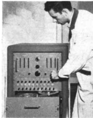
Vic-Dar System comprises a portable recording unit and a digital readout translator. The system can be used to accumulate and reduce data on speed, pressure, motion, temperature, etc.
