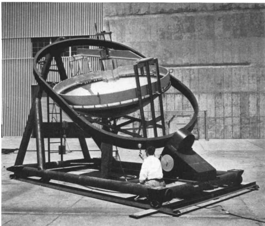
SOLAR FURNACE at Convair laboratory in San Diego, Calif., has a 120-inch mirror. The temperature is controlled by advancing or retracting a cylinder around the focal point.
