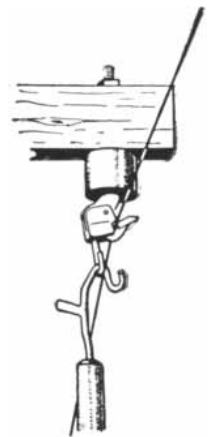
Key to the new "climbless" pole is this insulator. Ground crews use long-handled tools to place the wire in position and then lock it fast.
