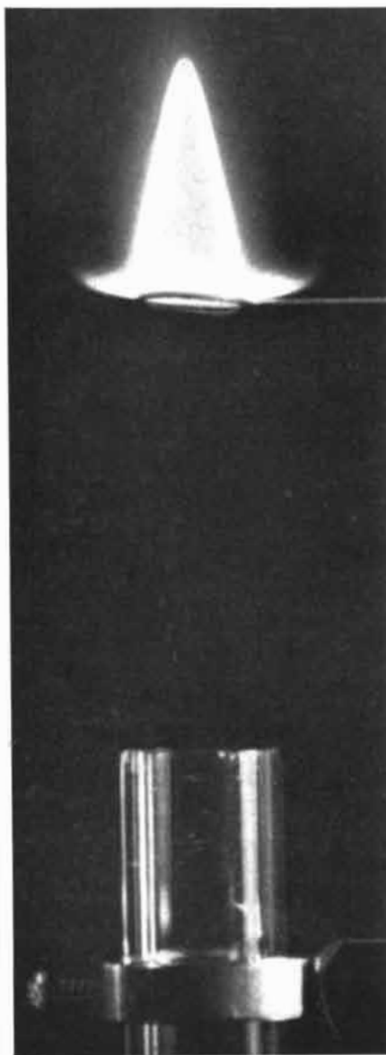
UPRIGHT FLAME CONE is stabilized on a ring placed in a stream of inflammable gas flowing from the glass tube at the bottom.
