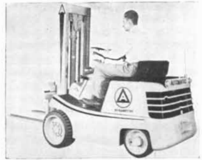
The generator and motor drive of the "Dynamotive" lift trucks built by Automatic Transportation Co. of Chicago are wound with silicone (Class H) insulation for protection against heavy overloads and excessive moisture. Automatic Transportation engineers report that "silicone insulation is used because it contributes to longer life and can take harder abuse than other insulating materials. Since we adopted it 7 years ago, we have never, to our knowledge, lost a motor due to insulation failure." No. 85
