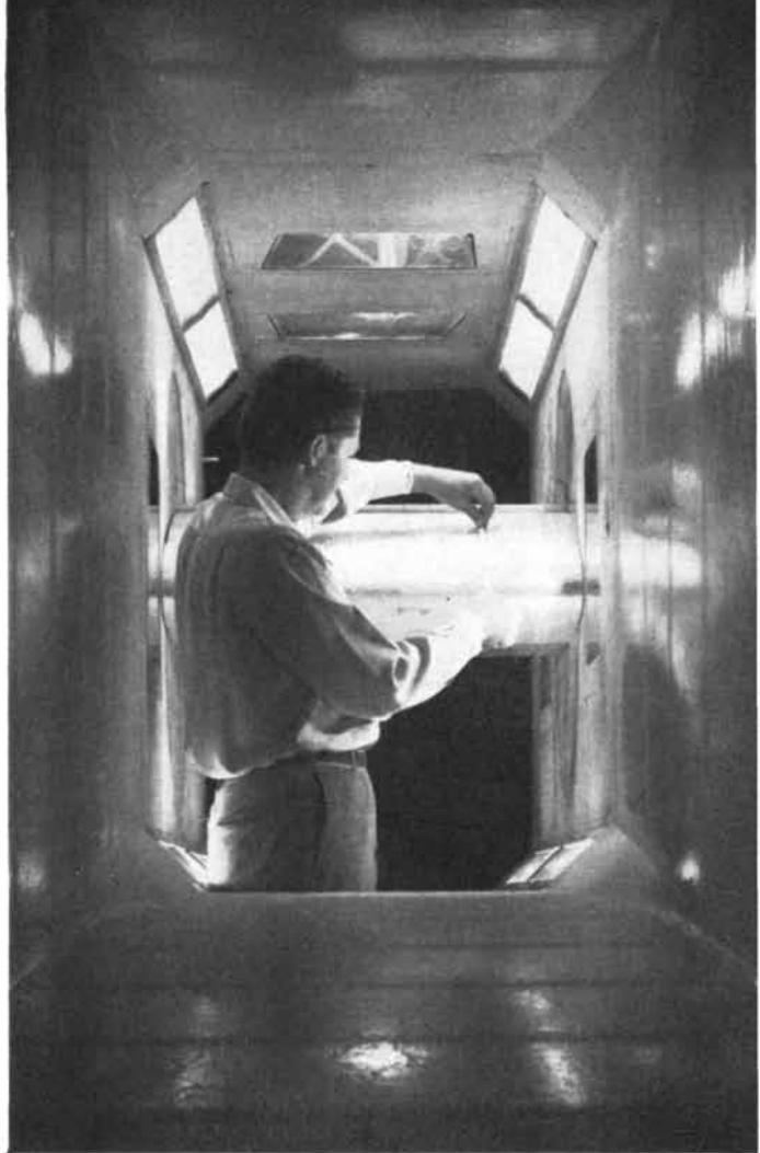
C. H. Fish , design engineer assigned to the tunnel, measures impingement limits of ice on C-130 wing section. The tunnel has refrigeration capacity of 100 tons, provides icing conditions of 0 to 4 grams per cubic meter, droplet sizes from 5 to 1000 microns.
