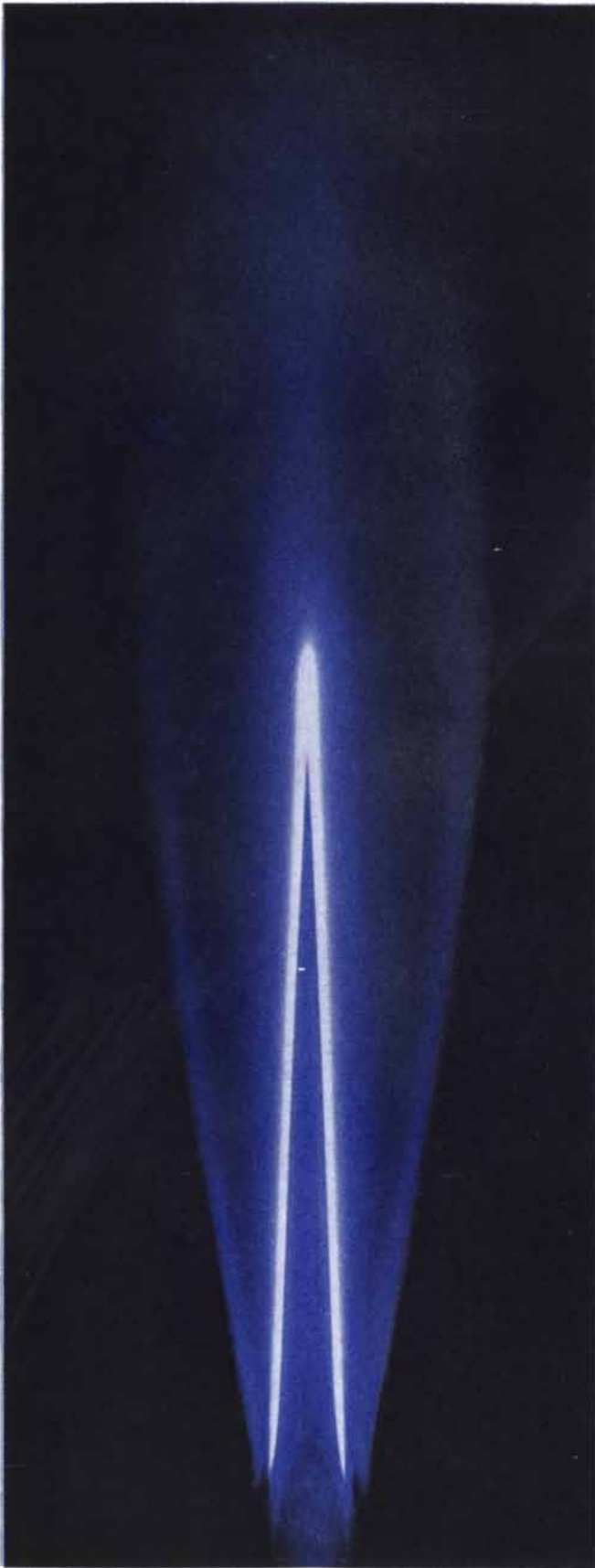
LAMINAR FLOW produces a flame with a tall, thin zone of primary combustion. This zone is the bright area in the center of the flame. The dark area within the bright one is the unburned fuel mixture; the blue area outside it, the zone of secondary combustion.
