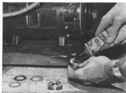
Providing 10 or more times the life of organic grease in high temperature motor bearings of the plain or shielded type, Dow Corning 44 Grease makes permanent lubrication a practical reality in sealed bearings operating at temperatures from —30 to 350 F. No. 84
