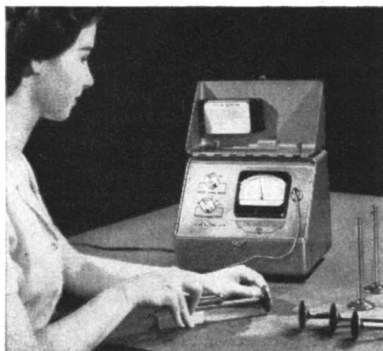
SURFINDICATOR is portable, easy-to-use, can be set up wherever 115 volts a.c. is available.
