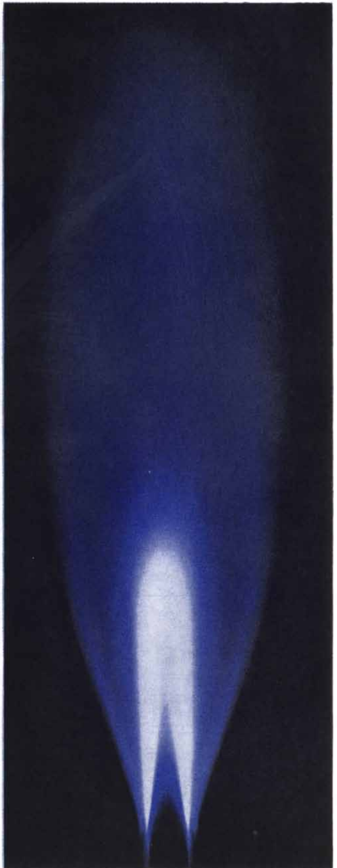
TURBULENT FLOW produces a flame with a short, thick zone of primary combustion. This permits more compact combustion chambers because the fuel burns in a shorter distance. Photographs are by S. Hight and R. W. Mascolo of Princeton University.
