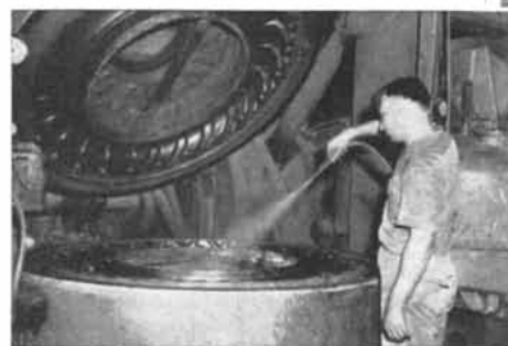
Relative inertness and incompatibility coupled with a high degree of resistance to breakdown at molding temperatures have made silicone mold release agents standard equipment in the rubber and plastics industries. Unlike organic mold lubricants, silicones cannot decompose at operating temperatures to form a carbonaceous residue on mold surfaces. No. 81
