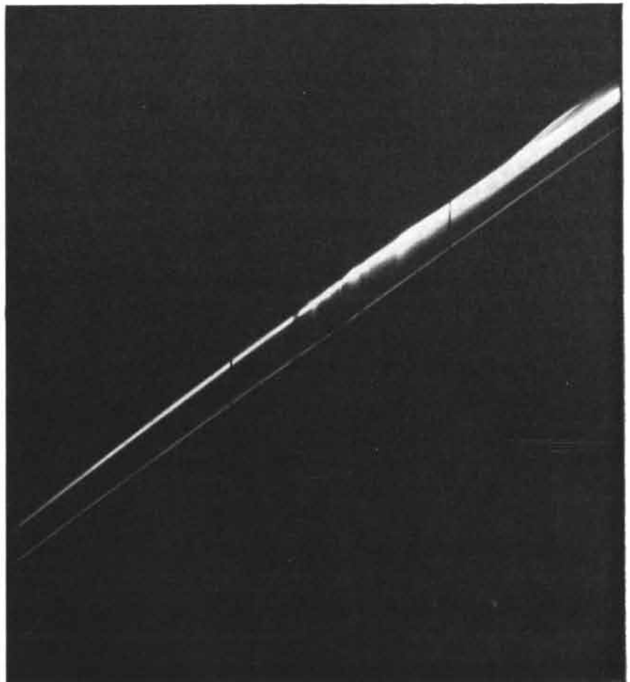
DRUM-CAMERA PHOTOGRAPH shows changes in the luminosity of argon after a shock wave has passed. The image of the luminosity is diagonal because the film in the camera was moved vertically. The thin line at the bottom represents the shock front; the thicker line above it, the luminescent gas. The dark zone between them shows the incubation period.
