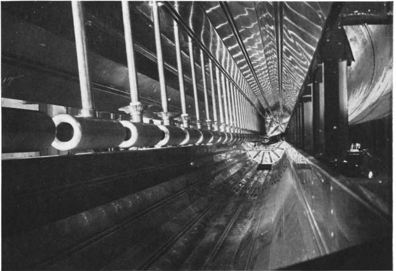
BERKELEY ACCELERATOR of the internal drift-tube type is shown with the resonator cavity open. Supports locate the drift
