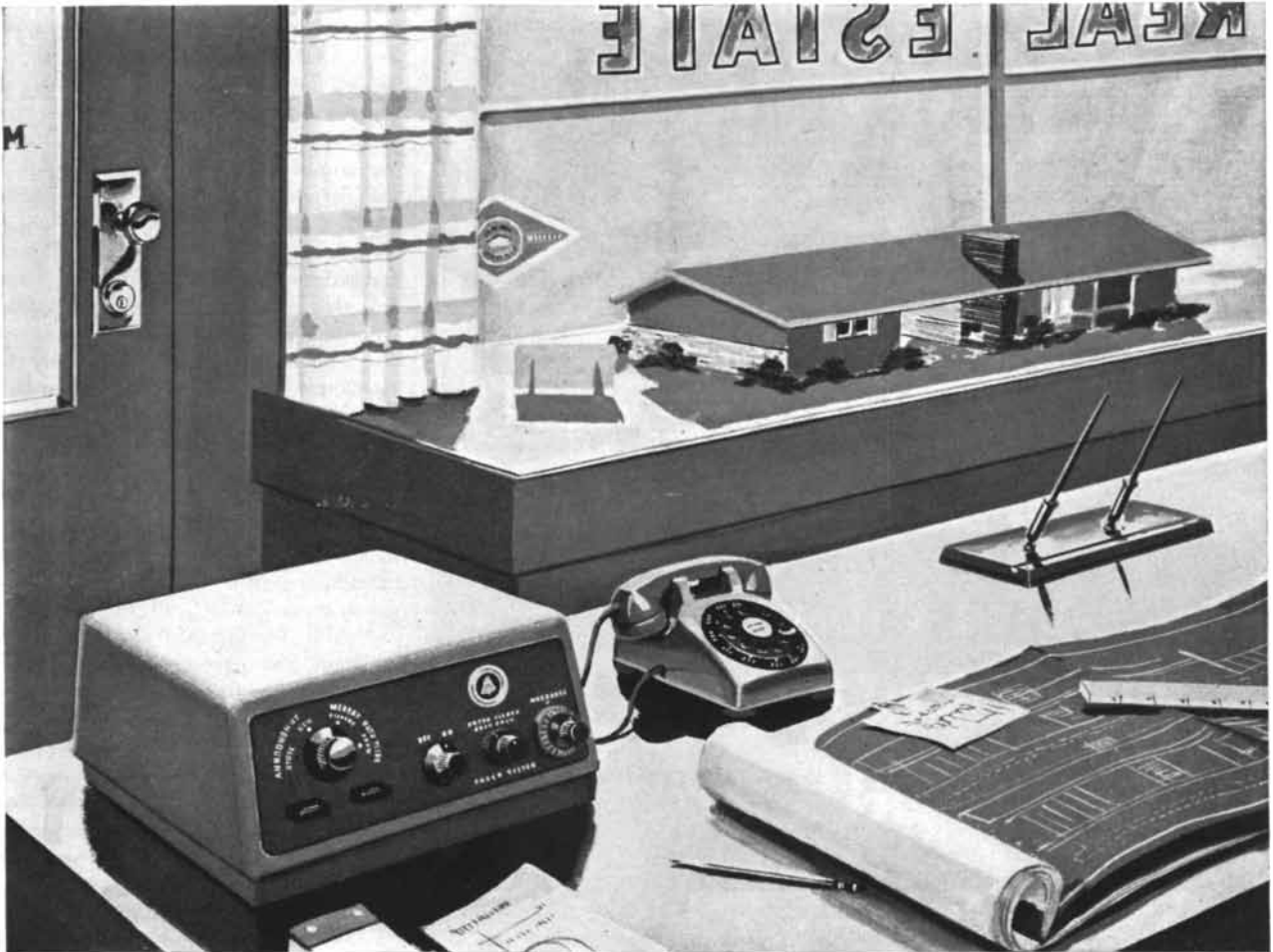
Bell's new Telephone Answering Set. In use, the machine tells the caller when to start talking, and when his time—thirty seconds—is up.
