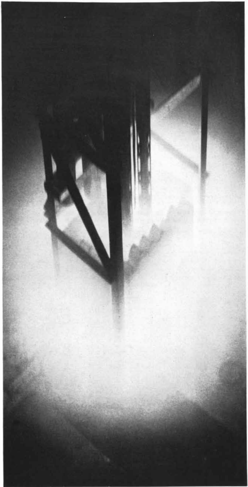
REACTOR CORE of an experimental "swimming pool" reactor illustrates the principle of pressurized water design. Plates of uranium-aluminum alloy are separated by ordinary water which serves as moderator and coolant. Above the plates are the suspended cadmium control rods. The diffuse light which surrounds the core is known as Cerenkov radiation.
