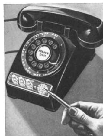
Pencil points to microphone in base of new telephone. Left-hand button controls volume, center one turns set "on" and lights up while in use. The third is an "off" button.
