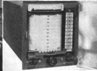
Horizontal scale above chart (left) continuously indicates control air pressure. Unitized construction (right) permits fast, easy removal and replacement of major sections.
