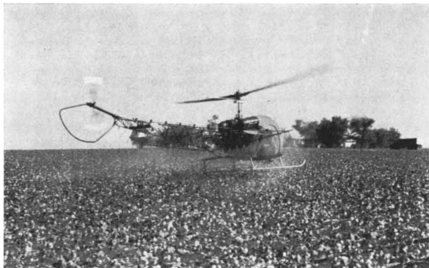
BELL 47G sprays defoliant on a cotton field near Plano, Texas, after which cotton bolls can be picked from the leafless plants by machine. The downdraft of the rotor aids spraying.
