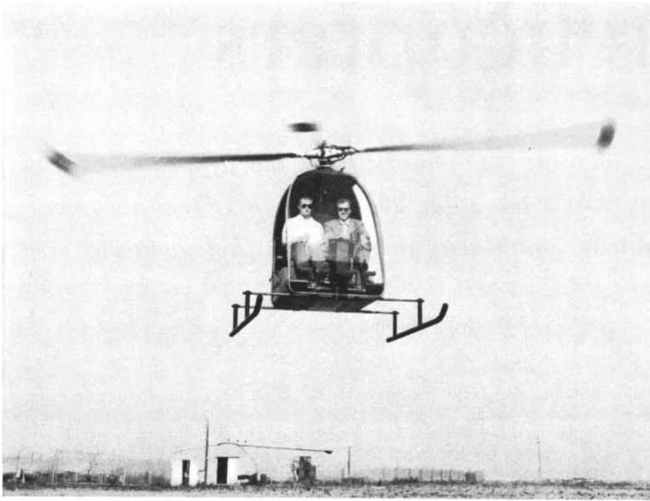
HILLER YHJ-1 has a novel propulsive arrangement. At the tip of each blade of its main rotor is a small ramjet. The high fuel consumption of the ramjets limits the cruising range of this machine.
