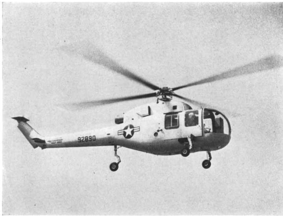
SIKORSKY S-59, which bears the Army designation H-59, is propelled by a gas turbine. It holds the three-kilometer speed record of 156.005 miles per hour and the altitude record of 24,500 feet.
