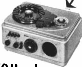
Durez take-up drum on "Srens" Wire Recorder Dictation Machine made by Crescent Industries.
