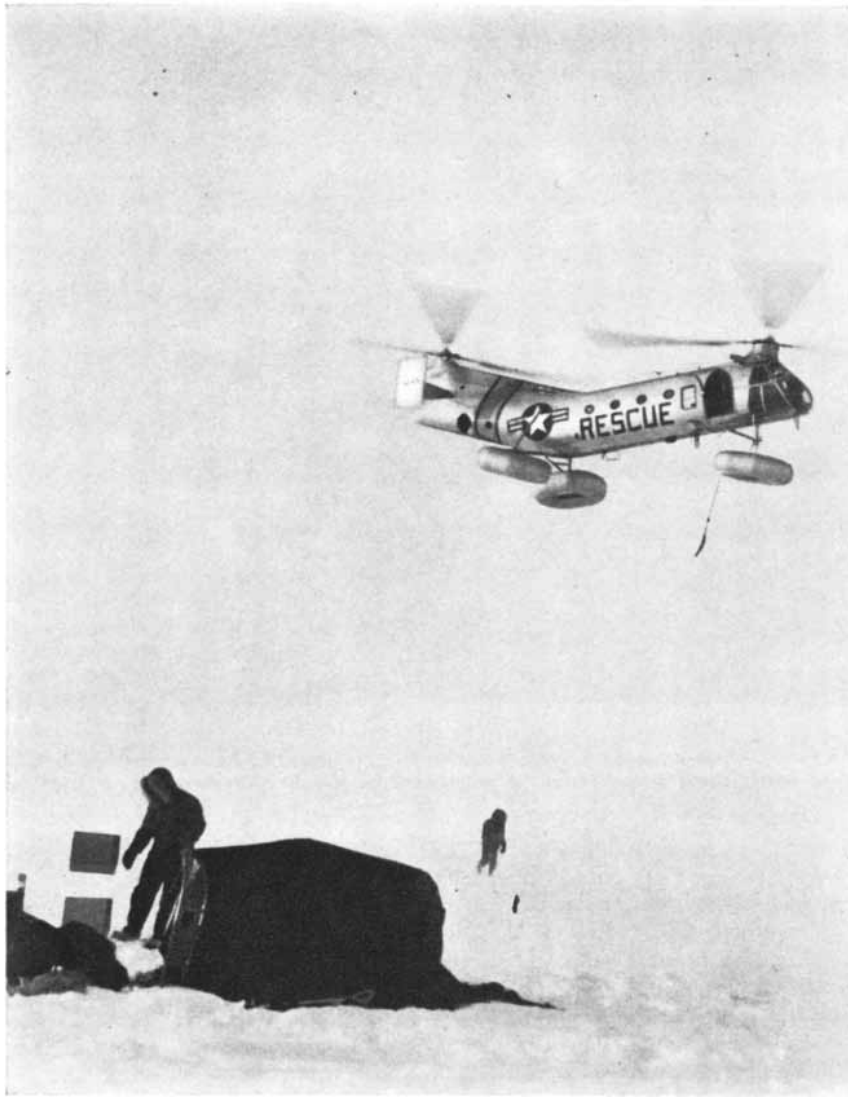
PIASECKI YH-21, especially equipped for Arctic operations, lowers a sling to a "survivor" during simulated rescue operations conducted on the Greenland ice cap near Thule Air Base.
