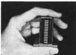
MAGNETIC HEADS for recording several channels of data on a single tape.
