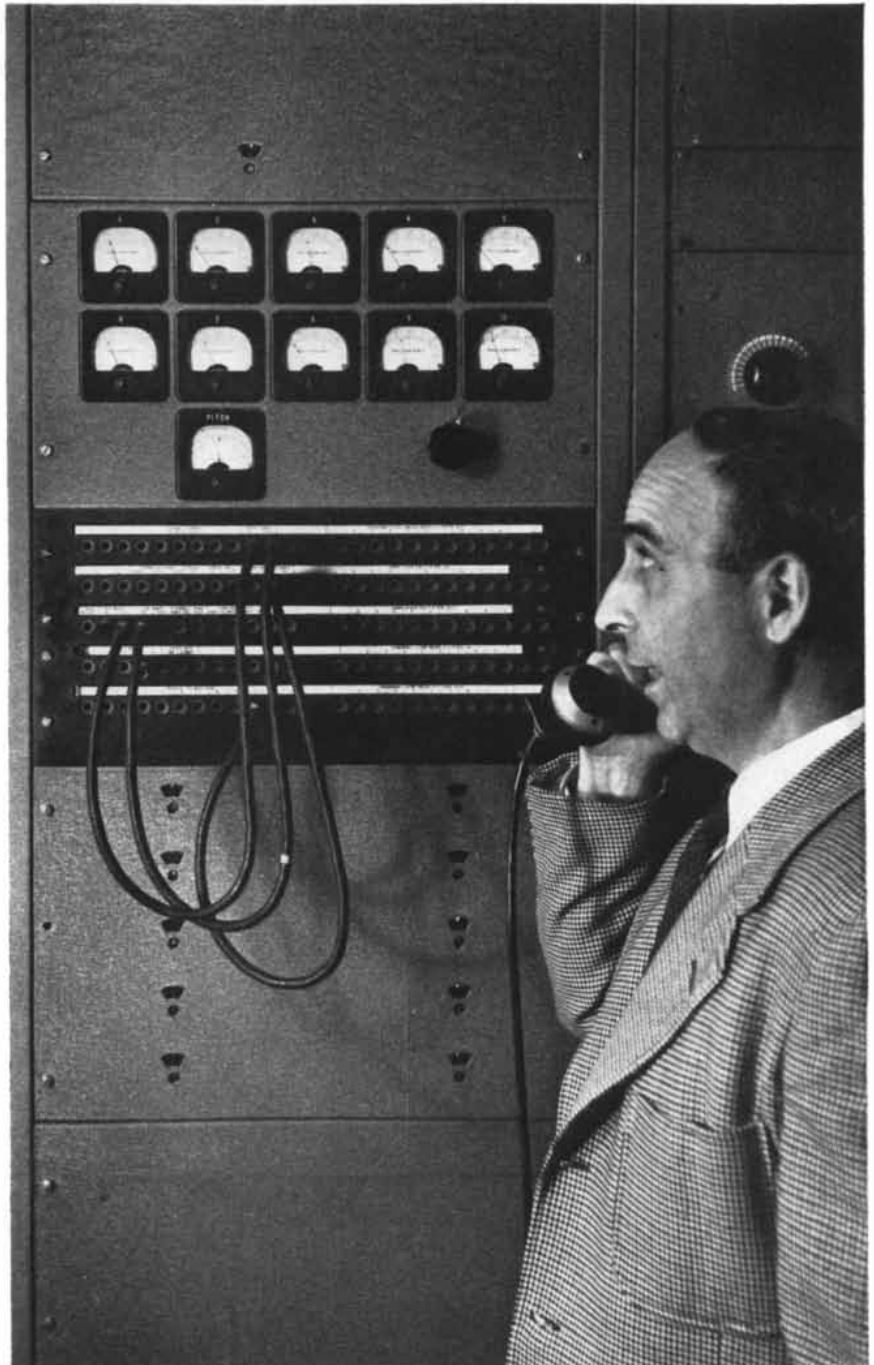
VOCODER is operated by Ralph Miller, its chief engineer. His voice, which has a frequency range of from 200 to 3,600 cycles per second, is compressed by the machine into a frequency band only 300 cycles wide. The meters at the top analyze the sound energy.
