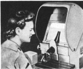
Pen point being inspected on an inexpensive bench model Jones & Lamson Optical Comparator. J & L makes a complete line of 11 Comparators, in both bench and pedestal types.
