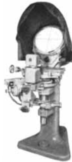
Pen point being inspected on an inexpensive bench model Jones & Lamson Optical Comparator. J & L makes a complete line of 11 Comparators, in both bench and pedestal types.
