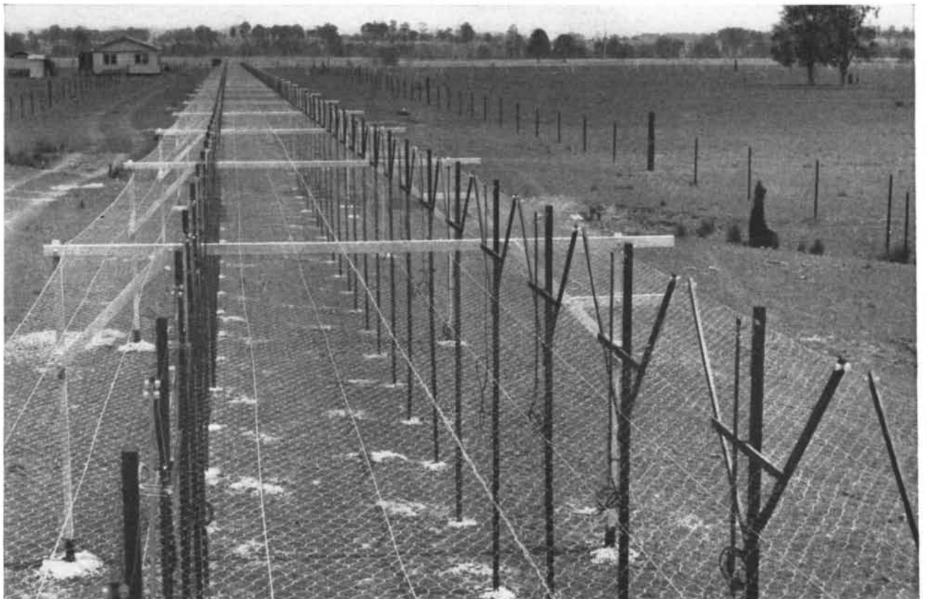
Larger telescope near Sydney has 600 dipoles mounted above a chicken-wire reflector 1,500 feet long.
