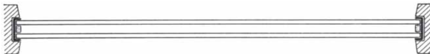
GLASS PANEL for a curtain wall, seen in cross section, has two panes which enclose a partial vacuum. It is 51 per cent more effective as a heat insulator than a single pane.
