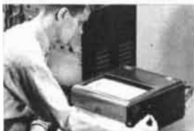
PORTABLE OSCILLOGRAPHS simplify field testing and development work—simultaneously record up to six channels of data.
