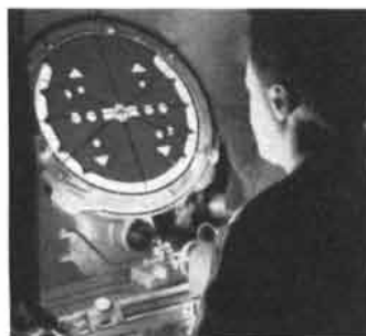
Punched holes in radio tube micas being inspected on a Jones & Lamson Optical Comparator. J&L makes a complete line of 11 Comparators, in both bench and pedestal types
