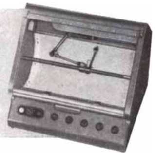
Librascope X-Y Plotter and Recorder; automatically displays data derived from punch cards, mechanical or electronic computers or sensing elements; features rapid graphic 2-axis display with provision for 10-fold scale expansion and zero suppression. Used in aero-dynamic and electronic research, as well as in mass data reduction systems for business and industry.
