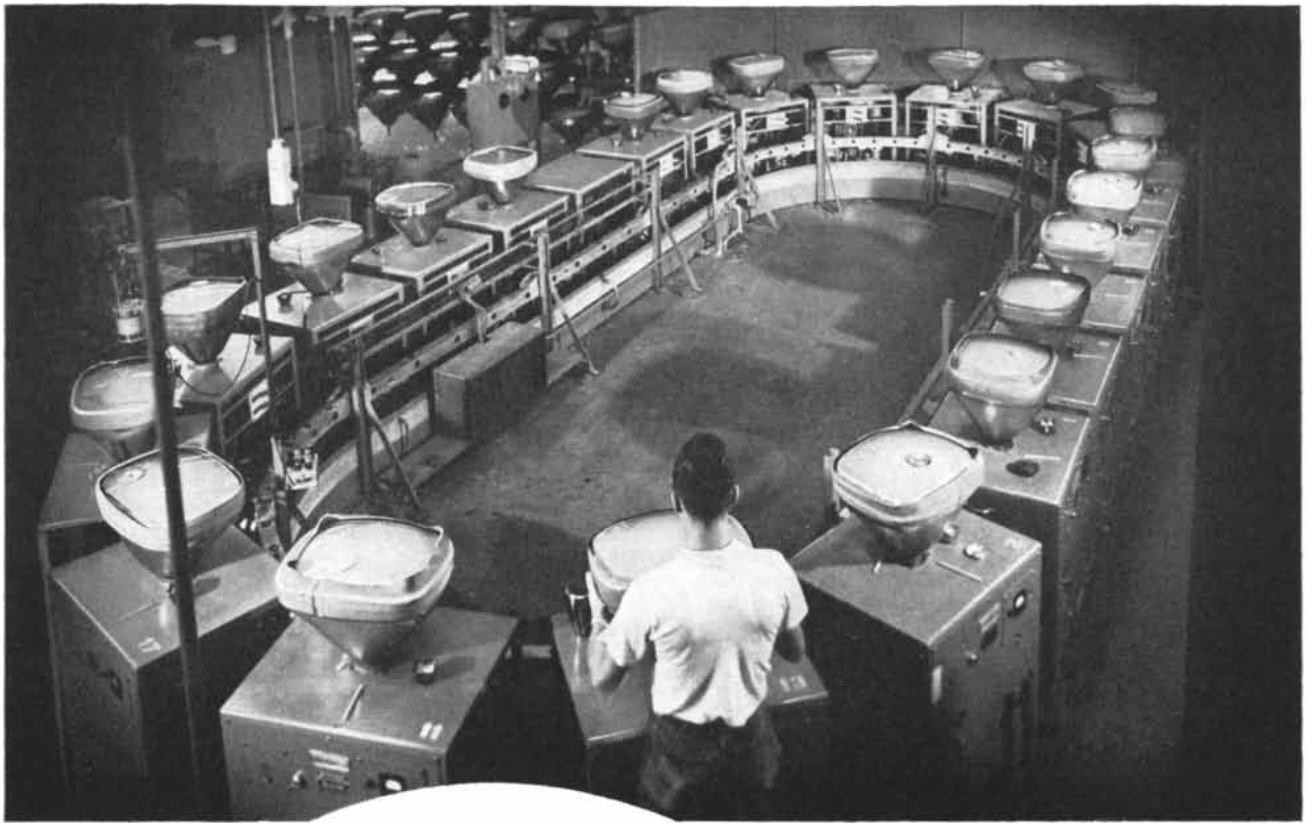
Overall view of Stokes continuous vacuum metallizing dolly system for aluminizing TV tubes at RCA's Marion, Indiana, plant. Operator is required only to load and unload tubes from the carts.
