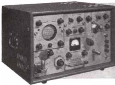
Kearfott X-band Test Set, frequency range 8,500 to 10,000 MC; a unique all-purpose portable radar test set, comprising a power monitor, spectrum analyzer, wave-meter and signal generator which supplies an accurately calibrated signal of known level with variable amplitude and pulse-width combinations. Also provides FM, square wave and CW output.
