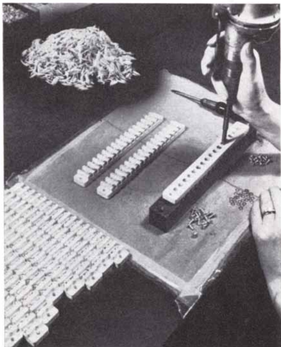
TERMINAL BLOCKS WITH EXCEPTIONAL STRENGTH , both electrical and mechanical, are being molded for the U. S. Navy from Cyanamid's new MELMAC® Molding Material 3135, shown in the inset. A unique melamine-glass high-impact molding material, MELMAC 3135 has very high arc and flame resistance. It can be compression- or transfer-molded into small or large parts, can be preformed and preheated, and flows so well that intricate and thin-sectioned parts can be molded without "shorts." (No. 5)
