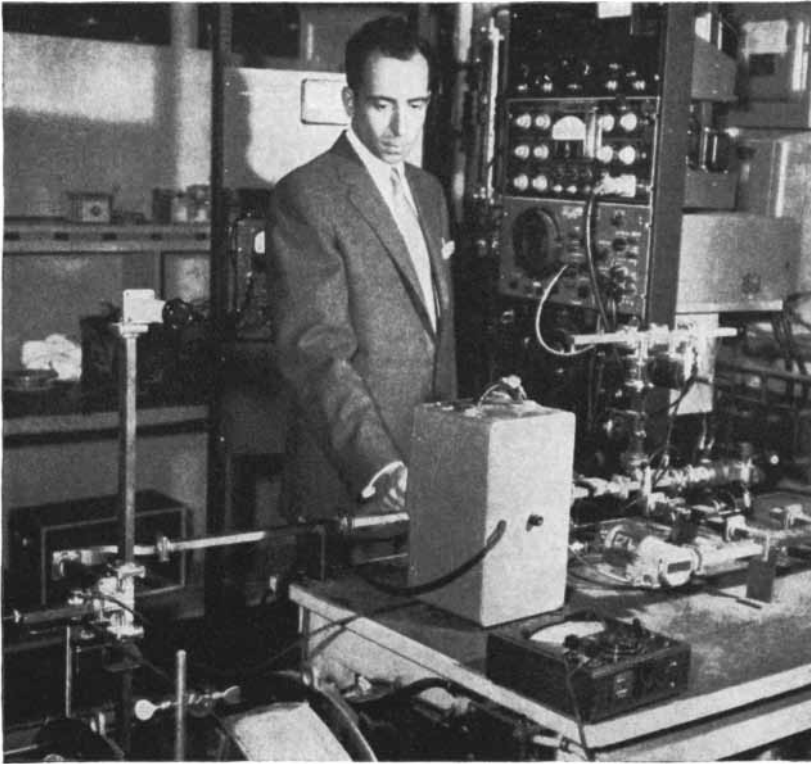
Studying ferromagnetic resonance. A cavity perturbation method is used, in which a ferrite specimen placed in a high Q microwave cavity changes cavity properties in accordance with electrical and magnetic properties of the material.
