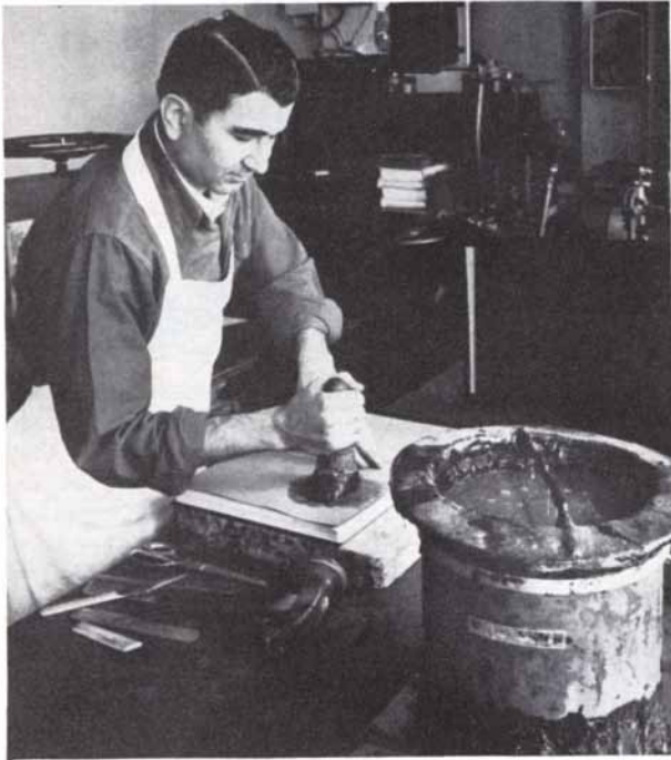
ANIMAL GLUES STAY FLUID FOR DAYS with less than 1% of Cyanamid's Dicyandiamide (based on dry solids) added as the fluidizer. This non-progressive property imparted by dicyandiamide, a property many other fluidizers lack, means glues stay workable and spread smoothly for days, give better results, cost less. (No. 3)
