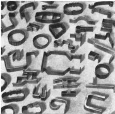
Fig. 3. Roll forming produces an almost unlimited variety of shapes.
