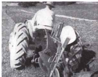
Tractor tires are made with BUTYL because BUTYL gives low tread wear and high resistance to weather, cracking, cutting, and chipping.
