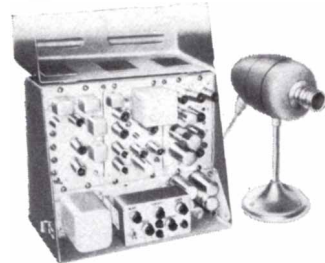
The "Bullet" TV Camera; for industrial, institutional and educational use. Produces useful pictures under conditions of poor light; feeds any TV receiver or monitor; unique packaging permits placement in ordinarily inaccessible areas; unitized construction with plug-in component chassis minimizes maintenance requirements.
