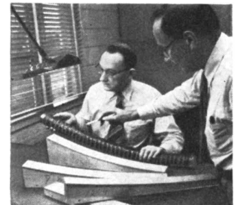
New type waveguide is bent on wooden forms for study of effect of curvature on transmission. The waveguide itself is here covered with a protective coating.
