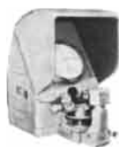
Checking a phonograph precious-metal needle for stylus projection, tip radius and included angle. Jones & Lamson makes a complete line of 11 Comparators, in both bench and pedestal types.
