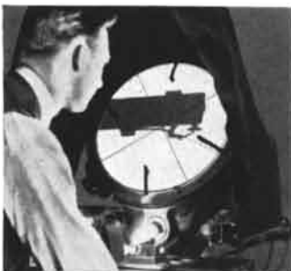
Checking a phonograph precious-metal needle for stylus projection, tip radius and included angle. Jones & Lamson makes a complete line of 11 Comparators, in both bench and pedestal types.
