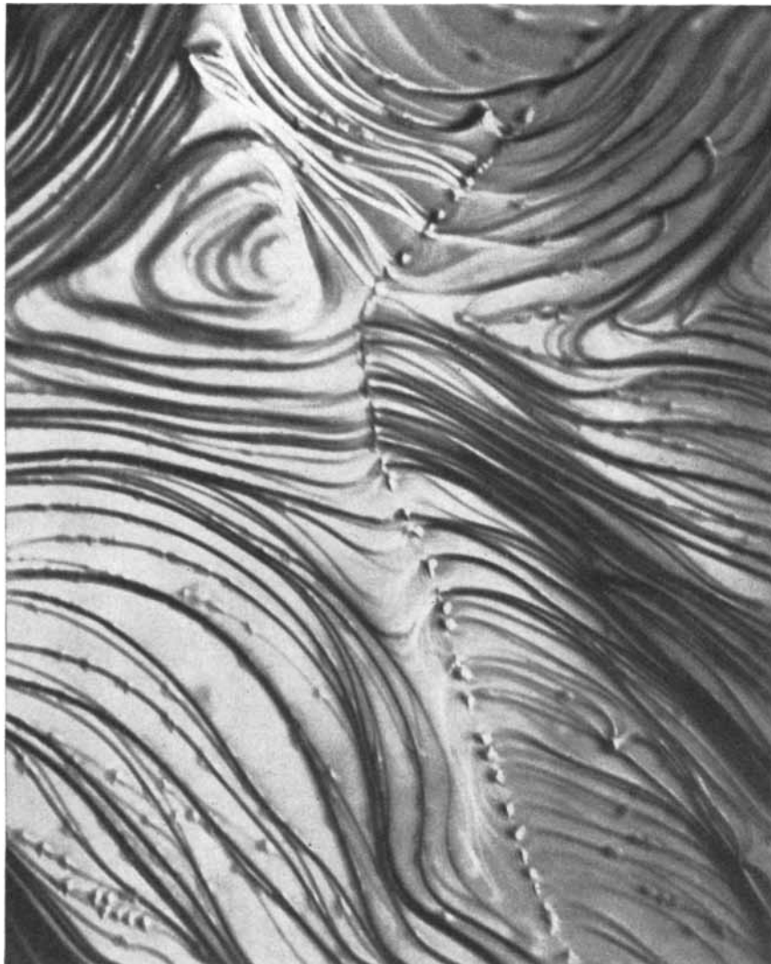
ACID ETCH PITS, which occur at dislocations, outline a boundary between grains of a polycrystalline metal. The spacing between pits depends on the angle between the grains.
