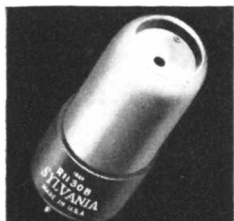
Sylvania Glow Modulator. Crater-glow, cold cathode type, used in facsimile and similar equipment. Light output may be varied by varying tube current.
