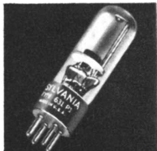
Sylvania Strobotron. Internally triggered, cold cathode tube which delivers light pulses of short duration. Used for study of rotary and reciprocatory motions.
