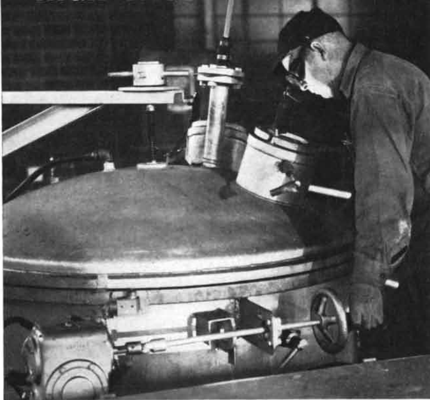
Technician viewing melt in NRC Vacuum Furnace from which come metals and alloys with new properties of strength, toughness, "cleanliness".
