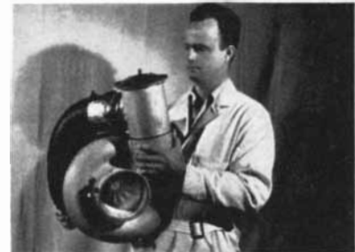
Mars gas turbine weighs less than 100 lb
