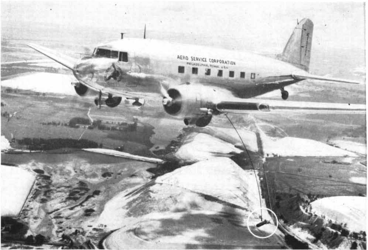
Airborne magnetometer survey, Johannesburg area. AERO crews are at work on six continents.
