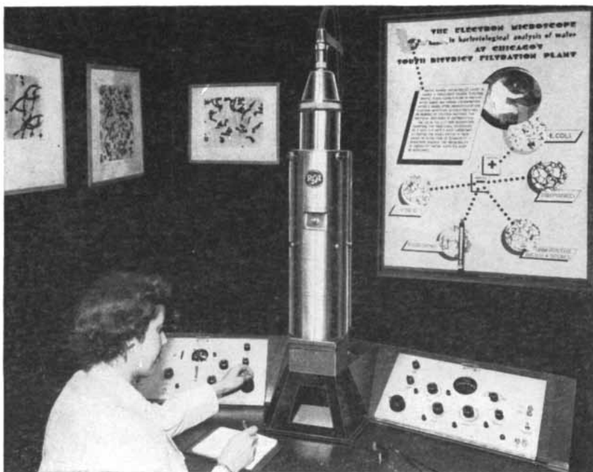
Technician at the Division of Water Purification, Bureau of Water, Chicago, Illinois, at the controls of the electron microscope.
