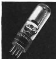
Sylvania Strobotron. Internally triggered, cold cathode tube which delivers light pulses of short duration. Used for study of rotary and reciprocatory motions
