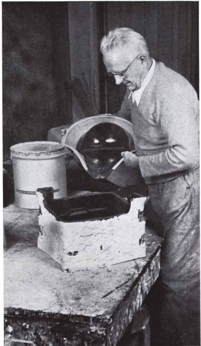
Top half or punch of drop-hammer die is poured. Epoxy resin with curing agent “sets up” in a few hours.
