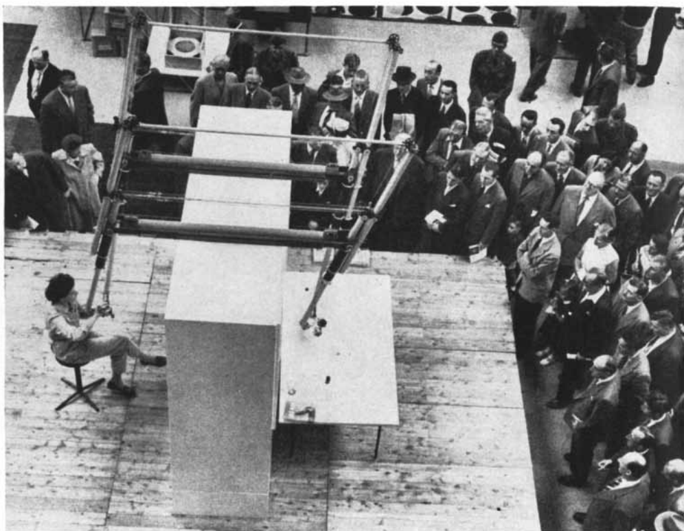
SLAVE HANDS, directed by woman on other side of wall, demonstrate their dexterity. In "hot" laboratories they enable chemists to handle radioactive material without exposure.
