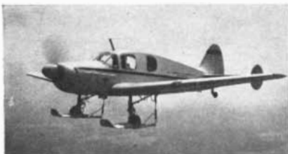
The hydro-lift landing gear developed by All American weighs less than 100 lbs., and permits a landplane to operate from virtually any surface.
