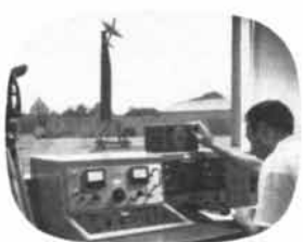
Antenna pattern study on radar search planes
