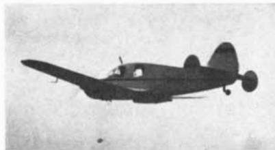
In flight the gear is retracted to fit snugly under the wing where it will have little effect on the performance of the airplane.
