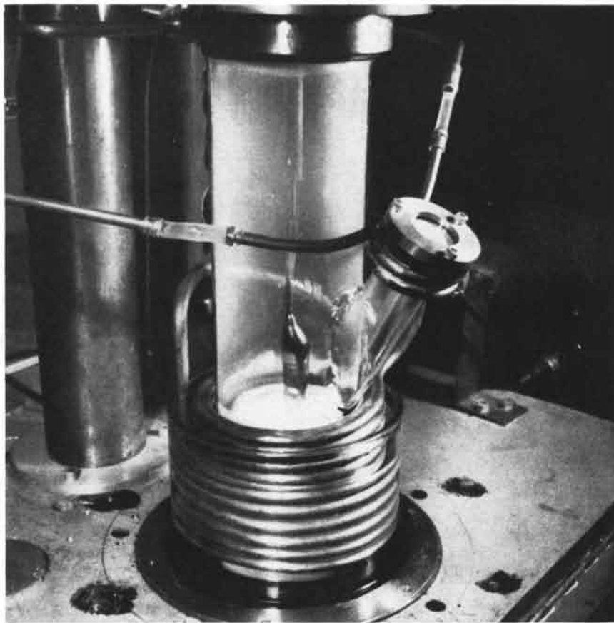
SILICON CRYSTAL is grown in a small induction furnace from a seed of pure silicon augmented by the molten material. Wafers for the battery are sliced from such crystals.
