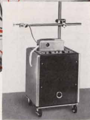
Brush Tension Analyzer records tension in the processing of filamentary materials.
