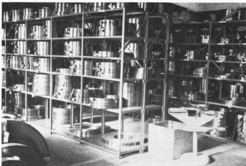
Highly polished steel, stored in this dehumidified room, is ready for immediate use. No costly, time-consuming cleaning operation is required, since the steel was completely degreased before it was placed in storage.
