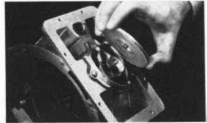
Dimensional stability, plus nonabrasive quality makes this glass ring a vital component in Sprague's planetary-valve gas meter.
