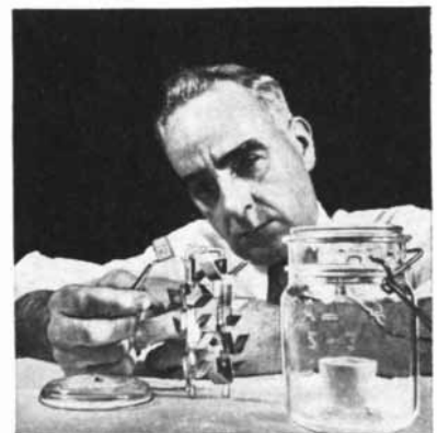
Through the study of thousands of specially cultivated whiskers, Bell scientists seek to prevent treacherous growths in telephone equipment.
