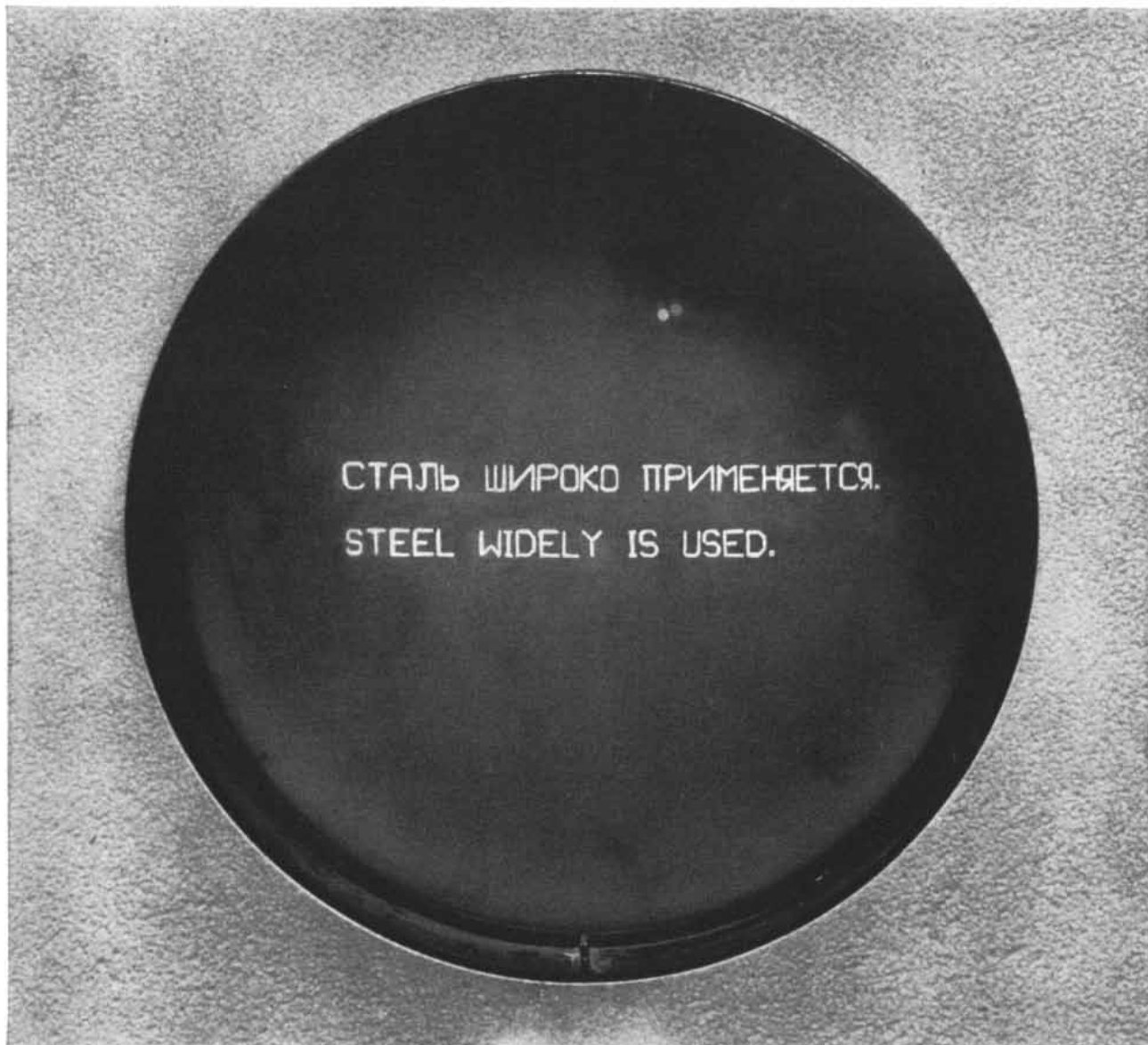
CATHODE-RAY TUBE displays three Russian words and their word-for-word translation. The tube is one output of Whirlwind , which was especially programmed to construct these symbols. Simi-
