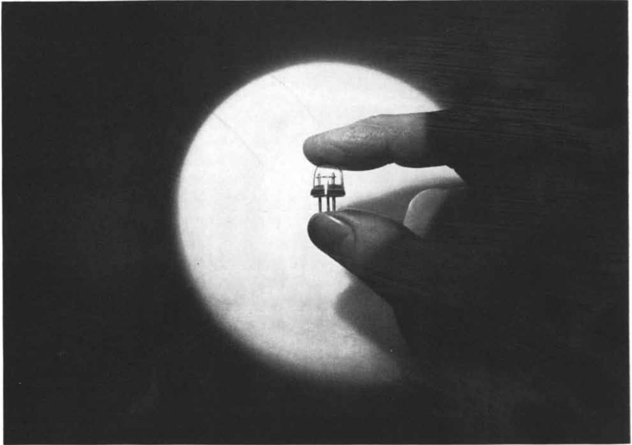
Experimental model of Bell's new high-frequency transistor. It has a cut-off frequency of at least 500 mc and can be used to amplify 2500 independent voices simultaneously.
