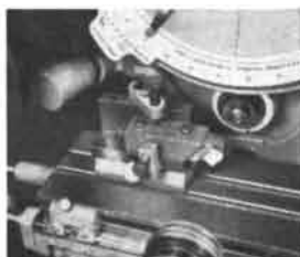
A J&L Comparator is used as a gauge to set and control limits of pre-set tooling for automatically controlled machining cycles.
