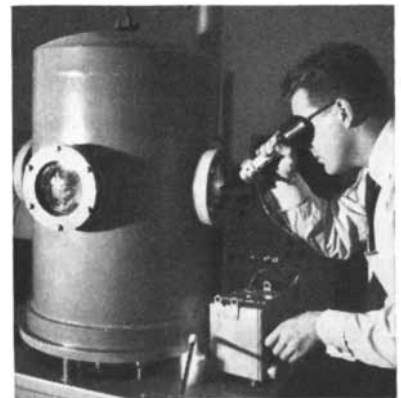
A Bell scientist checks temperature as arsenic vapor diffuses into germanium, creating 4/100,000 -in. layer.
