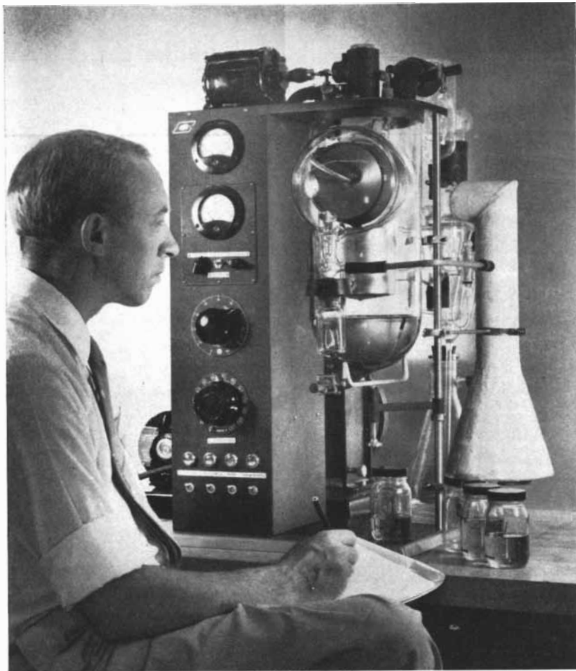
CMS-5 centrifugal molecular still. Distills heat-sensitive substances with molecular weight from 250 to 1200 at a distillate rate of .03 to 10 grams a minute.
