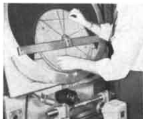
Inspecting location of ball contact points in steering worms, plus thread forms, solves a critical problem for the automotive industry.
