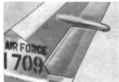
3 FIN BEAMS—High-strength, lightweight fin beams are made by CPT, using the world's largest flash-butt welder for assembly.
