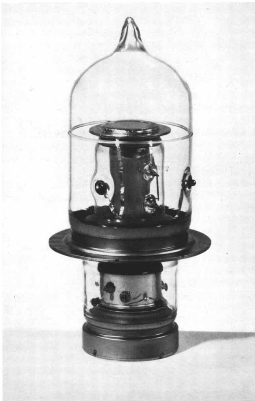
PILOT MODEL of the thin-film converter with a breakaway glass cap diagrammed on page 88 is shown in photograph. The tube was made by the Farnsworth Electronic Company.
