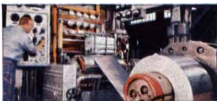
Reroll mill in separate aluminum section at a plant of The American Brass Company.
