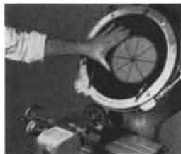
Checking keyway tolerances and hole diameter tolerances, as well as their locations and relationships to one another, in the same operation. Multi-base fixture allows rapid changeover for a variety of parts.
