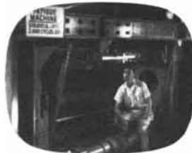
Fatigue test on Super Constellation skin
