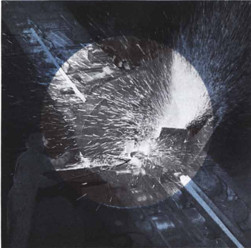
Sparks fly as a circular saw shears the end of a hot bar at Connors Steel Division plant, Birmingham, Alabama.
