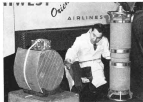
Industry's most versatile x-ray unit, the OX-175, is used to check oil cooler radiator. Cost of x-ray examination: $5.00. Previous mechanical inspection cost $40.00—and required removal of coring, thus shortening life of radiators.
