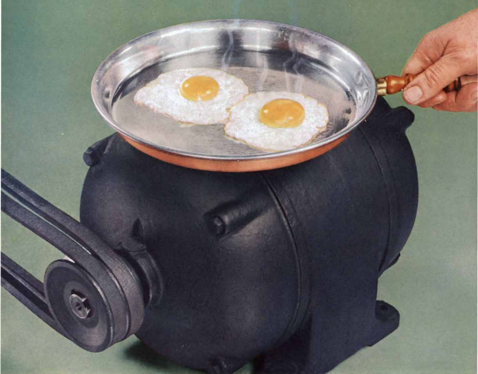
Laboratory motor is run at elevated temperatures to test heat-resistant characteristics of new magnet wire insulations.
