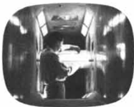
Hot-air cyclic de-icing test on radar search plane
