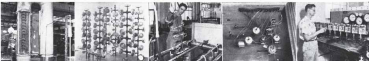
Most metals, subjected to severe cold forming, are susceptible to internal stresses. Each diaphragm and bourdon tube is heat treated to reduce internal stresses to a minimum.
