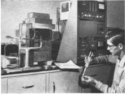
Uranium Ore Assay —Ontario, Canada. Uranium ore producers use Nuclear-Chicago scaling units in assaying various ore samples to determine uranium content.
