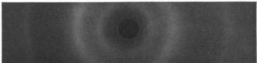
"X-ray" diffraction pattern showing halo effects denoting the amorphous structure of Kanigen
