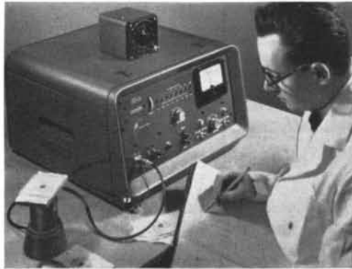
Industrial Research —New York, N. Y. Laboratory uses radioactive "dirt" and Nuclear-Chicago instruments to test washing machines, improve soil-removal techniques.
