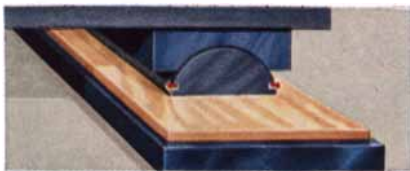
Arrows show direction of movement, as free end of approach roadway section slides on 8" x 17" phosphor bronze bridge plates.
