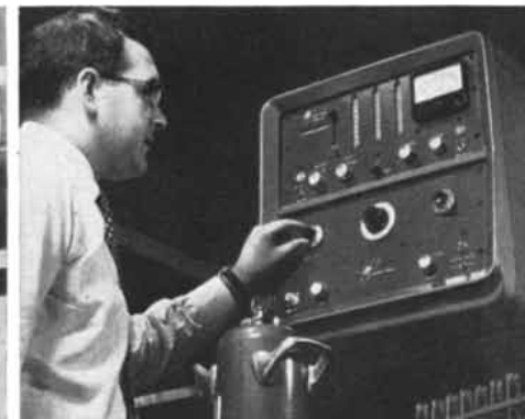
Gamma-ray Spectrometry —Chicago, Illinois. Radiation physicists study the energy spectrum of gamma emitting radioactive isotopes with Nuclear-Chicago spectrometer system.
