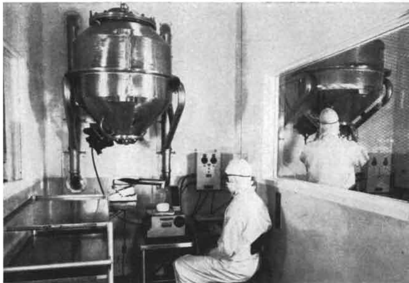
Sterile rooms at the Groton, Connecticut, plant of Chas. Pfizer & Co., Inc. are maintained at a constant low humidity—
