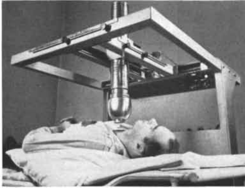
Medical Diagnosis —Detroit, Michigan. Nuclear-Chicago Isotope Scanner makes it possible for physicians to have "picture" of radioisotope distribution in organs of patient.
