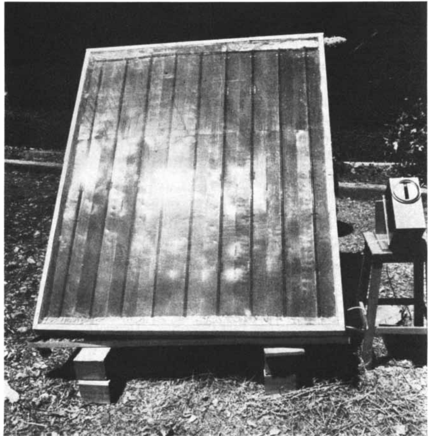
EXPERIMENTAL FLAT-PLATE COLLECTOR at the National Physical Laboratory of Israel traps solar energy between a reflector and transparent plastic. At right is a light meter.
