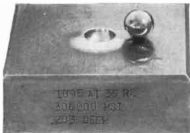
A Kennametal ball pressed to a depth of .203" into a 1095 steel plate of 35 Rockwell C hardness, under pressure of 306,000 psi
