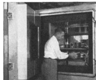
Ford Instrument Company engineer placing equipment designed for Navy instrument in one of the environmental test chambers.
