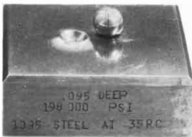
A steel ball cracked when pressed to a depth of only .095" into a 1095 steel plate (35 Rockwell C), under pressure of 198,000 psi
