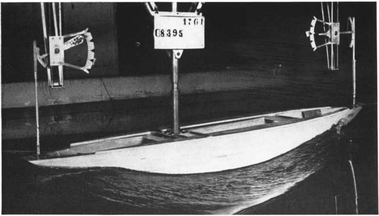
A model sailboat "runs before the wind" in the Experimental Towing Tank at the Stevens Institute of Technology
