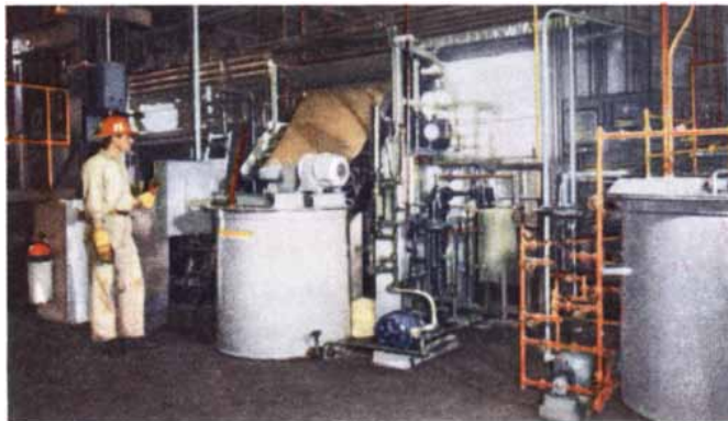
In pilot plant equipment like this, USS chemical engineers are developing and testing new processes for the recovery of new coal chemicals. Such pilot plant studies provide data for the design of commercial units for the recovery and synthesis of these chemicals.
