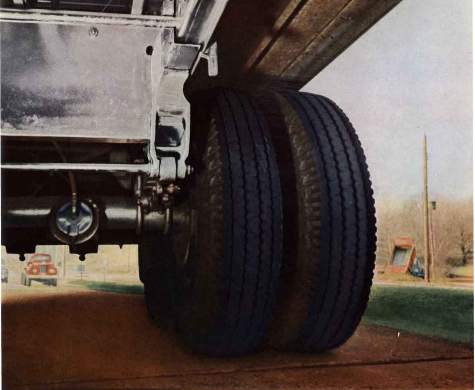
In balancing load, Trailmobile's shiftable wheel assembly slides along the main frame beams, forward or backward as needed.
