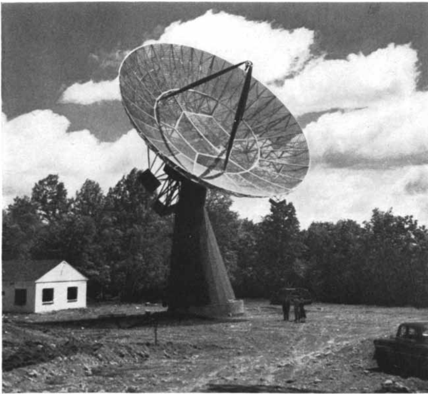
60-FOOT TELESCOPE of Harvard Observatory has equatorial mounting, which is preferred by astronomers but requires heavy counterweights, visible at left behind the reflector.
