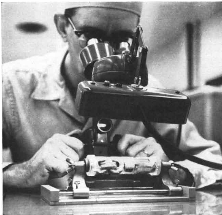
Even minute imperfections, visible only under the microscope, can disqualify repeater parts for use
