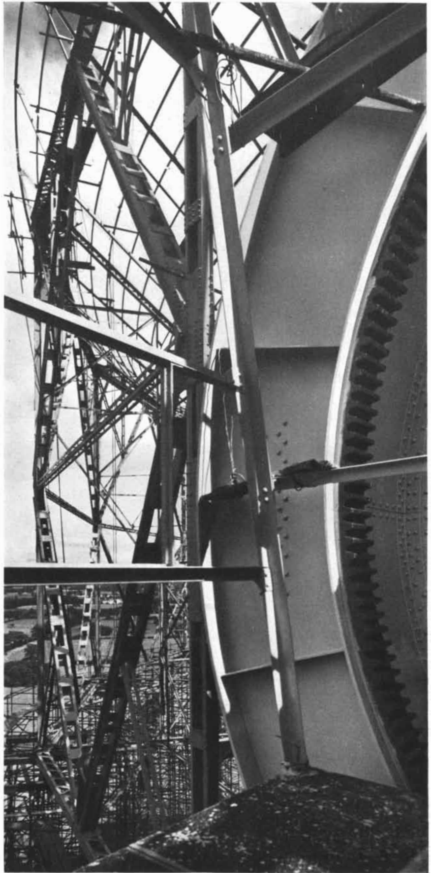
RING GEAR for vertical rotation of the 250-foot reflector is shown here. Entire telescope will be rotated horizontally by driving the wheels that bear the weight of the structure.
