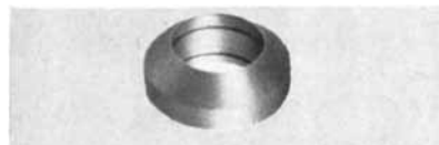
Kanigen-coated brass fitting
