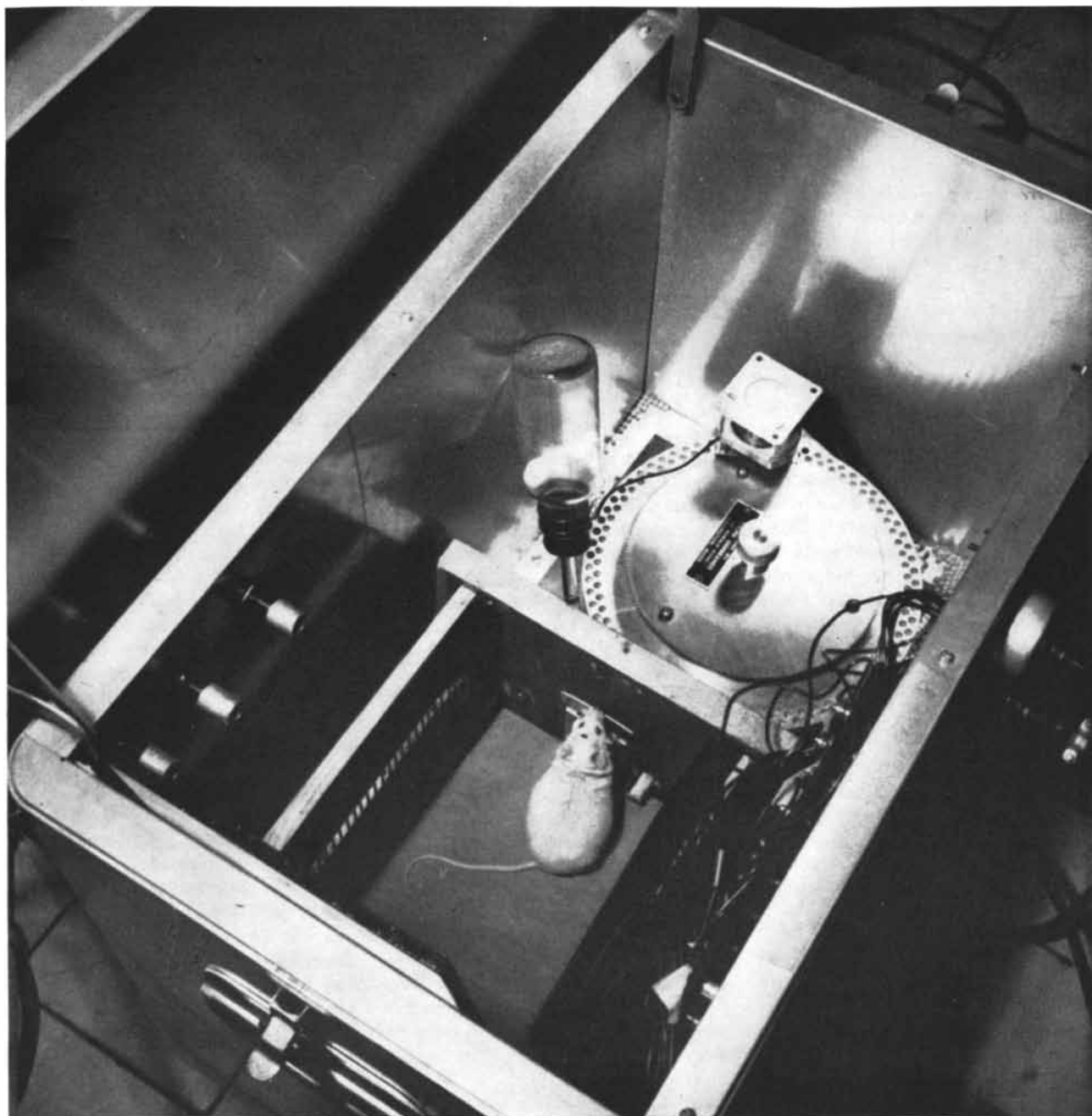
OBESSE MOUSE PRESSES A LEVER in a special cage designed to study the feeding behavior of small animals. The large disk at the upper right is part of an automatic feeder that discharges pel-
