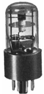
Sylvania Glow Modulators Crater-glow, cold cathode type, used in facsimile equipment. Light output varies with tube current. A modulation frequency range from 15-15,000 cps.
