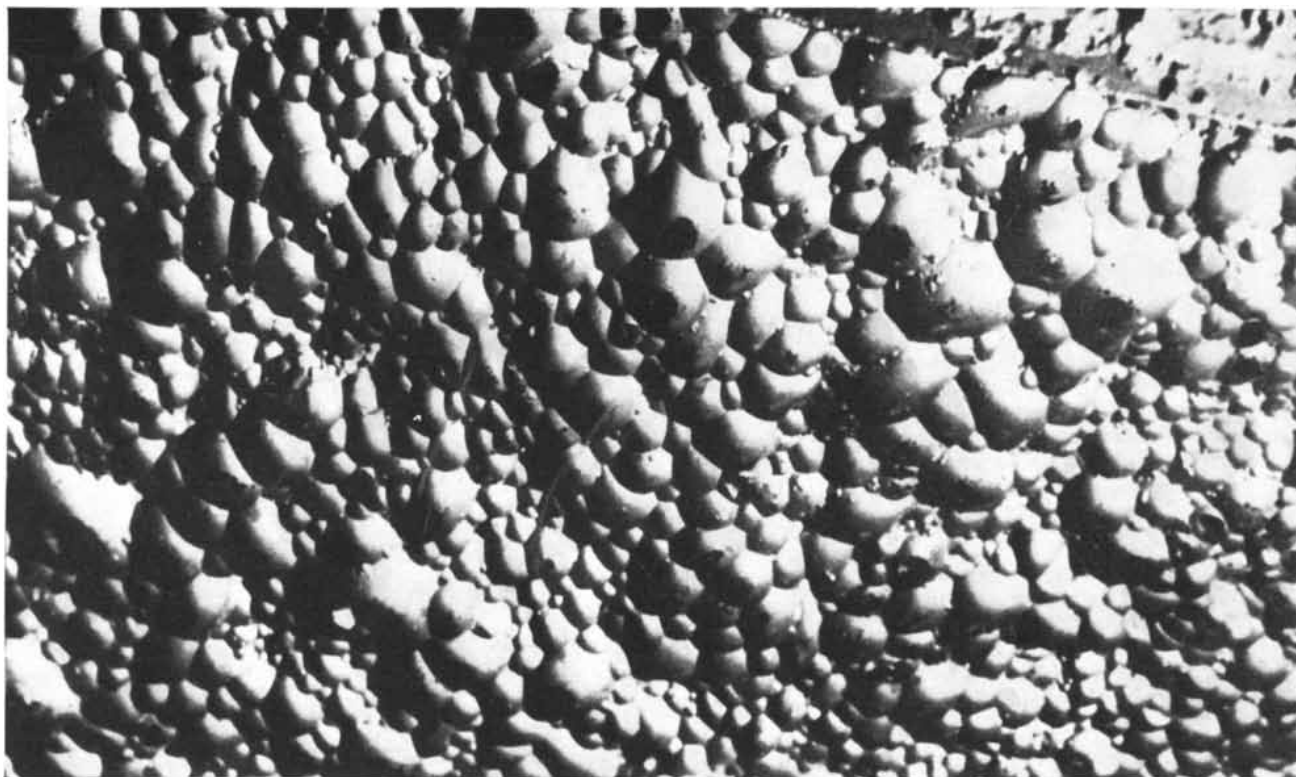
BUBBLES at the surface of a flotation cell are coated with mineral particles. This froth may now be skimmed off and the remaining so-
