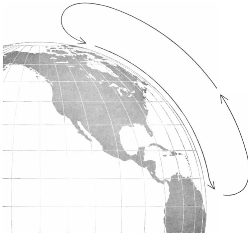
“CLASSICAL” CIRCULATION , predicted by older theories, shows air rising in the tropics, flowing north aloft, falling near the poles and returning south along the surface.
