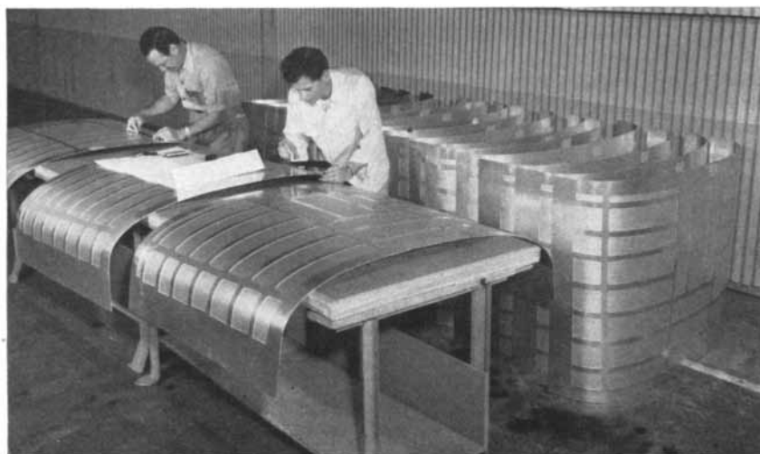
PARTS ARE CHECKED by inspectors after etching. The inspector at the right measures the depth of the etch with a micrometer. These parts are rear air ducts for the F-100 fighter.
