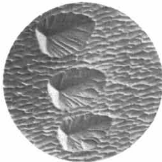
Aluminum grain showing sub-grain structure. Parlodian replica. Chrome shadowed.
