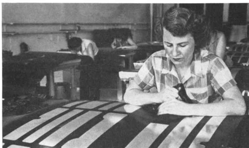
MASKANT IS PEELED from a part in the pattern to be etched. The maskant is cut in the pattern by scribing it with a sharp tool. This must be done without scoring the metal.
