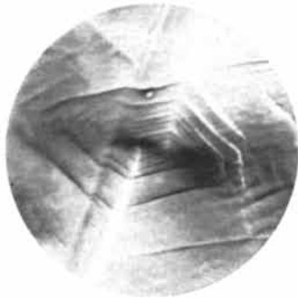
Aluminum grain structure, showing spiral dislocation. Parlodian replica. Chrome shadowed.
