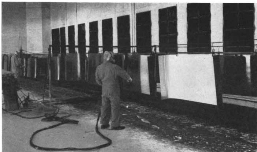
AIRPLANE PARTS ARE SPRAYED with maskant before they are etched at Downey plant of North American. The maskant, which covers the metal with a dark coat, is now baked.
