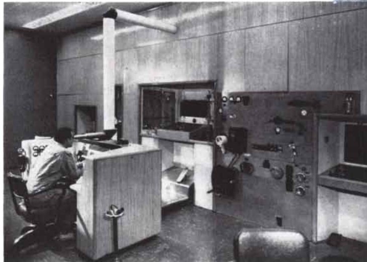
Operator at the control console of the RaLa processing laboratory. The apparatus shown at the right is seen through the periscope.
