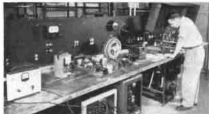
LOAD TESTING This power panel provides AC or DC in a wide range of currents, voltages, and frequencies . . . permits testing Ohmite products under operating conditions.
