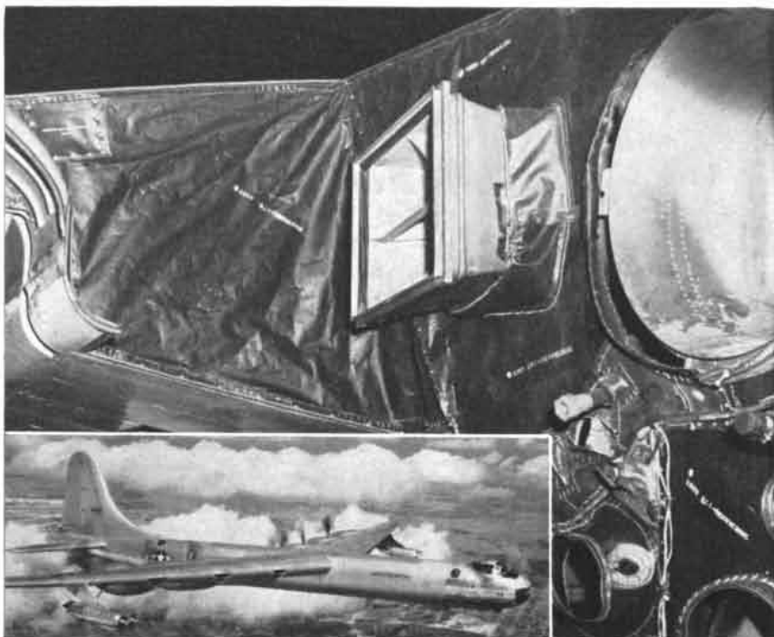
Fire-resistant Du Pont "Fairprene" lines engine-nacelle cleavage areas of Convair B-36. Lightweight, flexible elastomer permanently bonded to stainless-steel mesh adds strength to fire wall which readily conforms to complex contours.
