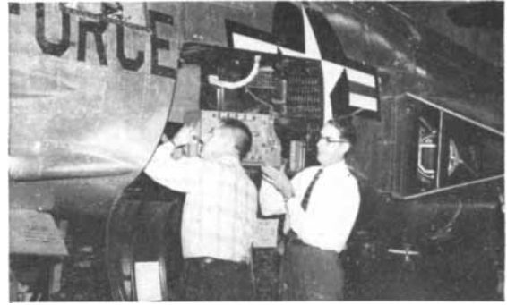
Kennard and V. C. McIntosh of WRIGHT AIR DEVELOPMENT CENTER Install Magnetic Tape Recorder in F-101 Aircraft.
