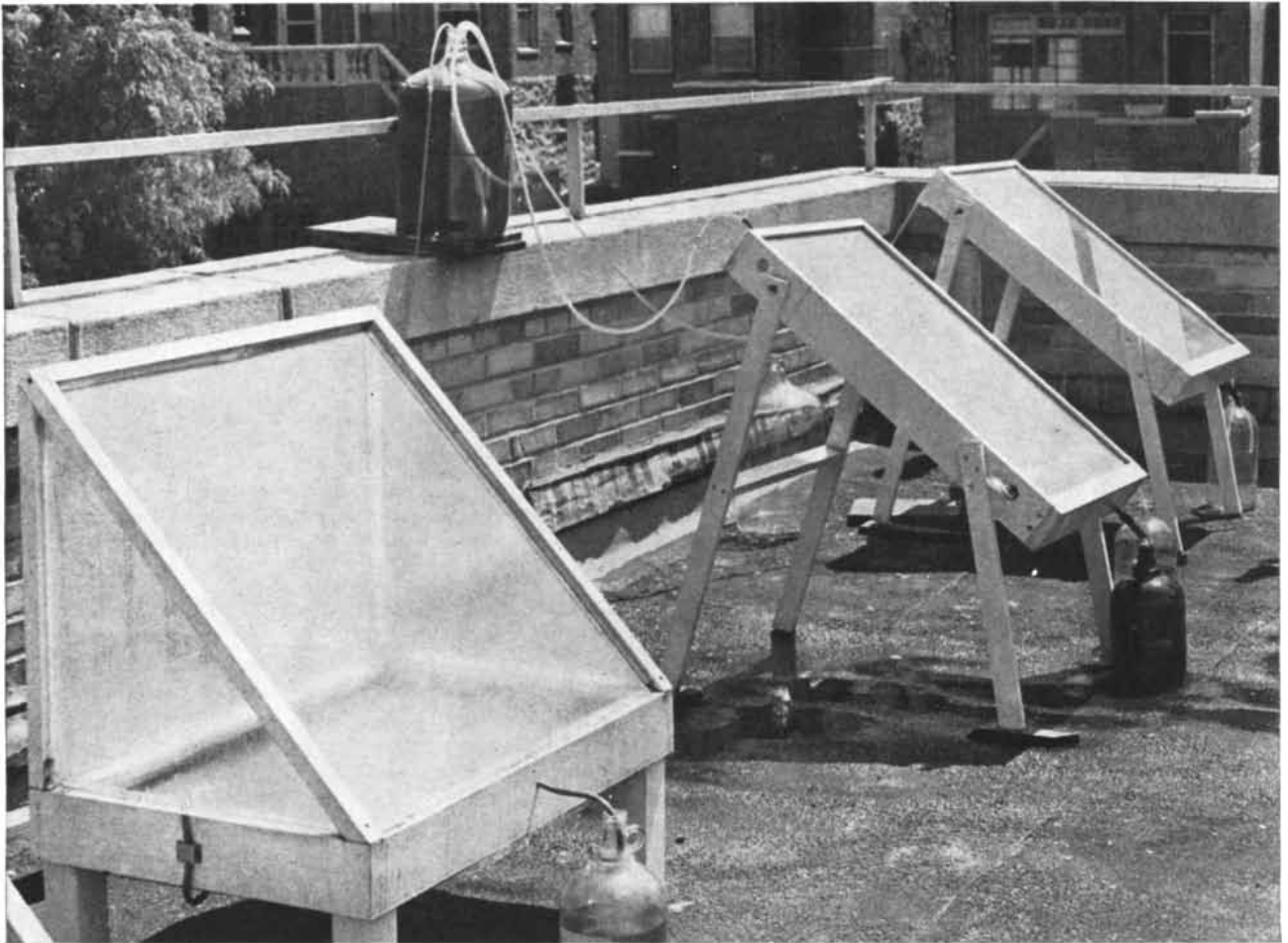
EXPERIMENTAL SOLAR STILLS designed by Maria Telkes are shown on rooftop at New York University. In unit at left water vapor rising from shallow pool of sea water condenses on under-
