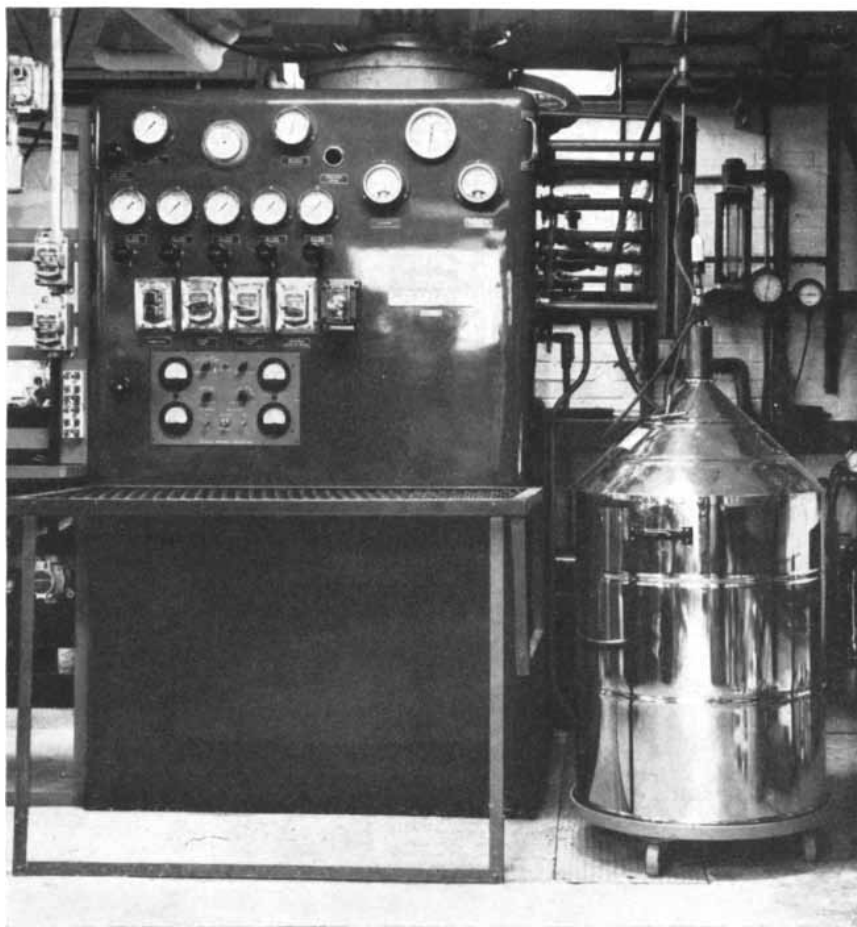
LIQUID HELIUM for the experiments at the National Bureau of Standards was made by this helium cryostat. The vacuum storage tank at right holds 20 gallons of liquid helium.
