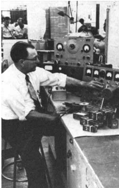
SERVO AMPLIFIERS used with a four-way electrohydraulic valve being tested by Douglas electronic engineer.
