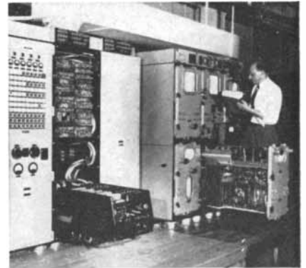
SPECIAL PURPOSE COMPUTERS , both analog and digital, comprise a great portion of the work at FICo. In both types, FICo employs a module technology which simplifies not only the problems of design and manufacturing, but servicing as well. This permits stocking fewer spare parts and allows easy training of personnel.
