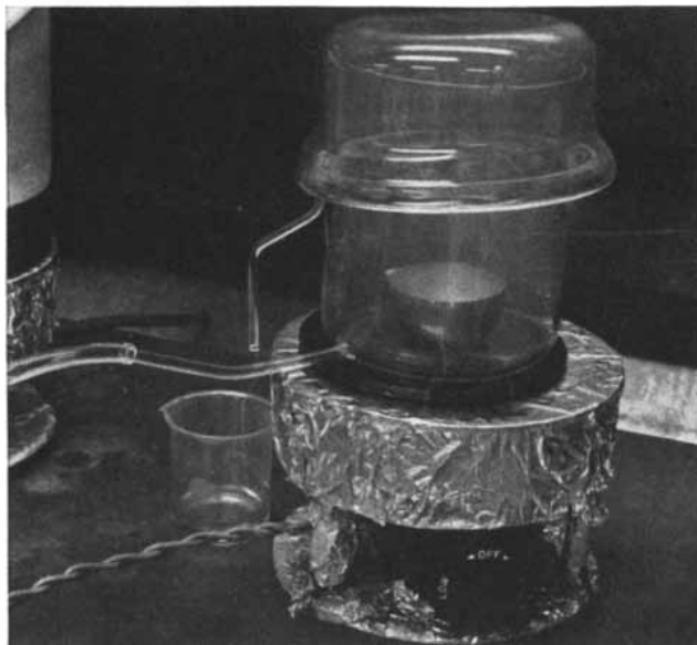
SAMPLE IS WEIGHED ( upper left ) before it is chemically broken down into its constituent elements. Pure water for the chemical manipulations is made by quadruple distillation ( upper right ).
