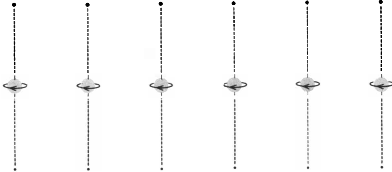
SPINNING NUCLEI of cobalt 60 (gray circles) emit electrons (large dots) preferentially in one direction along their spin axes and anti-neutrinos (small dots) in the other. The effect is ordinarily undetectable (top) but can be seen when spin axes are aligned (bottom).
