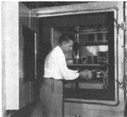
ENVIRONMENTAL TEST CHAMBERS like the one above are used by Ford Instrument Company engineers in many projects involving design and development of equipment to be used at extreme altitudes or temperatures. Instruments for jet engines, for polar navigation, and Army and Navy fire control are FICo products.
