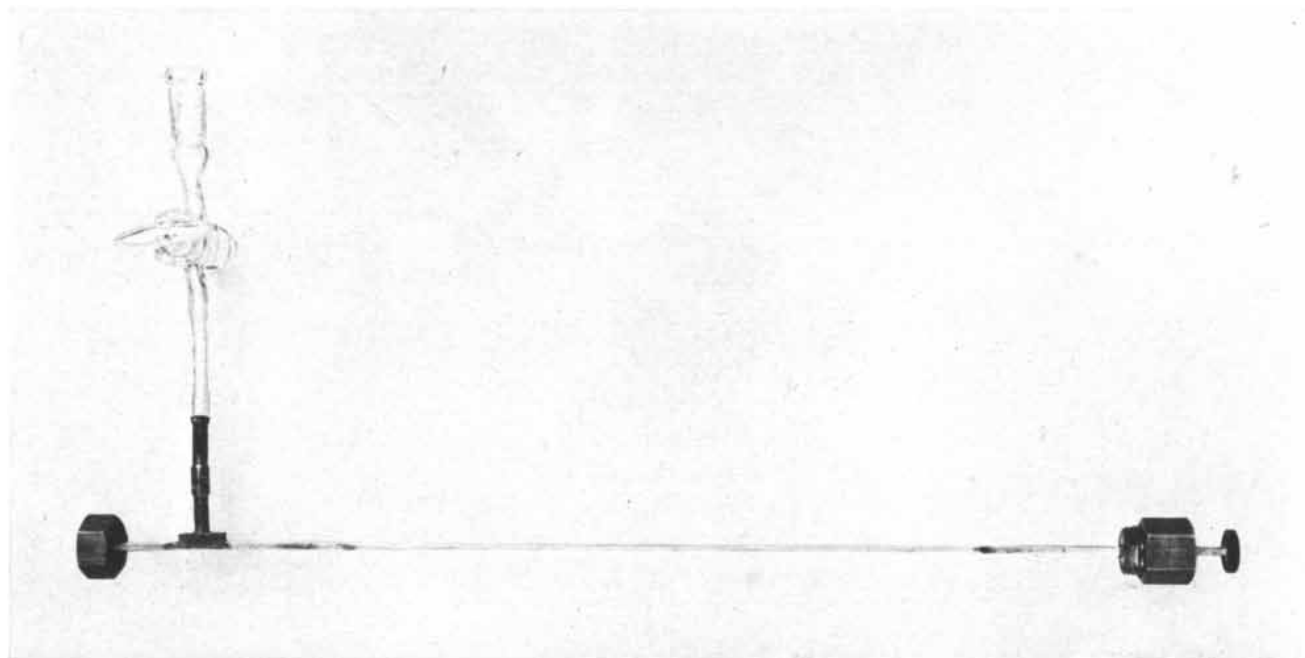
CRYSTAL AND CAT WHISKER at upper left, which are mounted at the end of the waveguide at the bottom of the preceding page,
