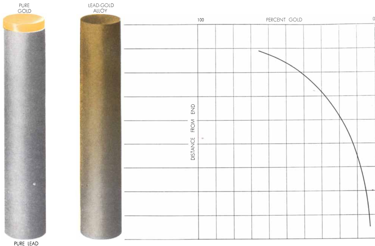
GOLD WAS FUSED TO LEAD (cylinder at left) and heated in an early diffusion experiment. The result (cylinder at left center) was that gold migrated down through the lead, and lead diffused into the gold. When the cylinder was cut into sections and analyzed, the sections at the top showed the highest concentration of gold. The curve shows how the concentration of gold decreased from the top.
