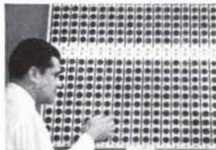
Converter Panels are designed to meet specific power needs, produce 80 watts of power per square yard of surface.
