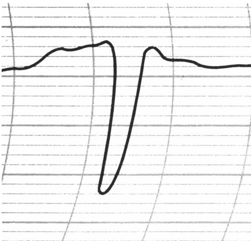
SPECTRAL LINE OF CYANOGEN BROMIDE, represented by a valley, has a wavelength of .87 of a millimeter. The frequency of this line is 345,837 million cycles per second.
