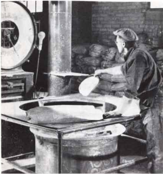
Each glass formula starts with the careful weighing of sands, clays and other specified ingredients. These are then thoroughly mixed and screened to uniform consistency.
