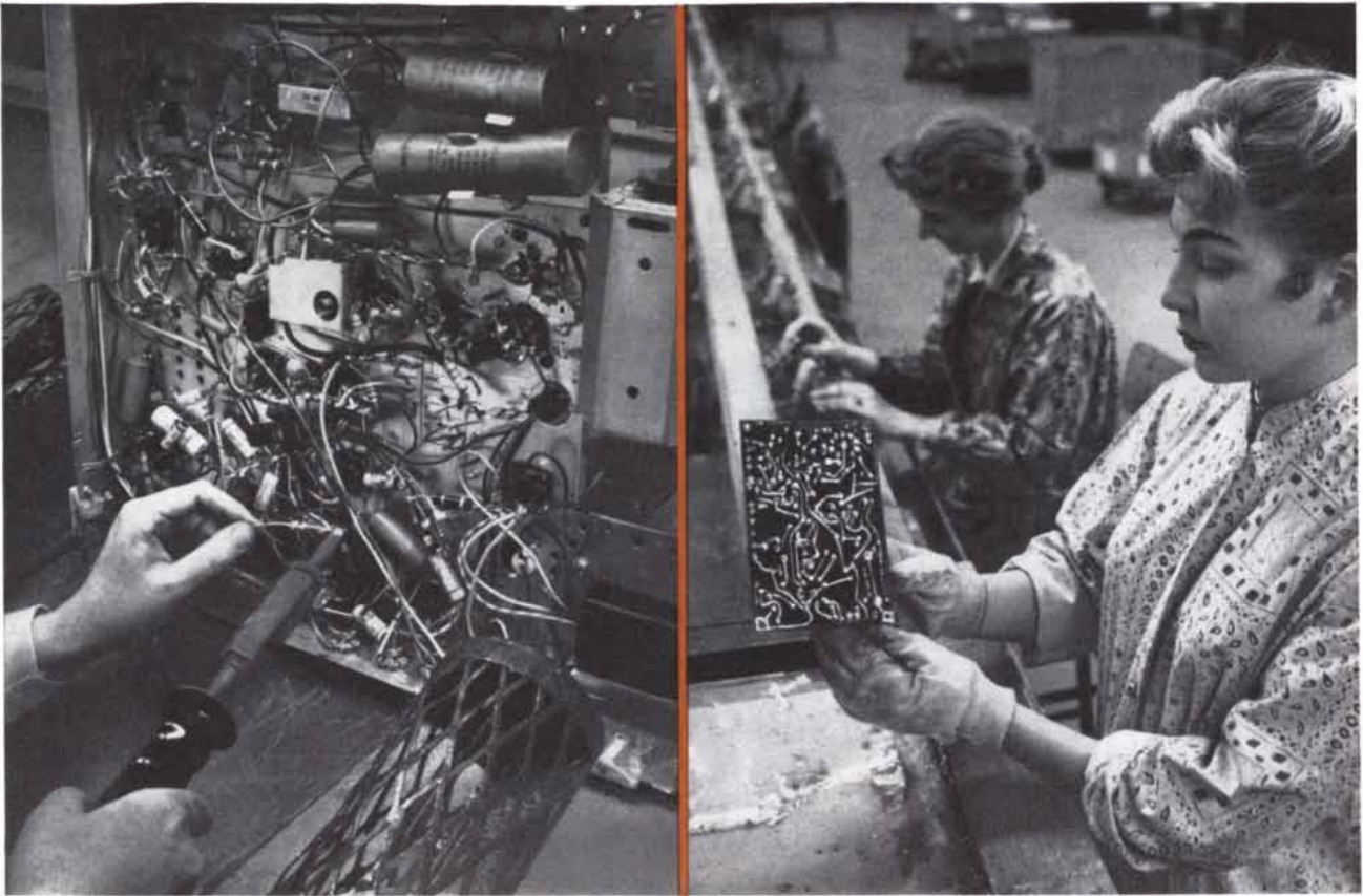
Old style hand-soldering has been replaced by faster, simpler dip-soldering in this modern plant of Emerson Radio & Phonograph Corporation.
