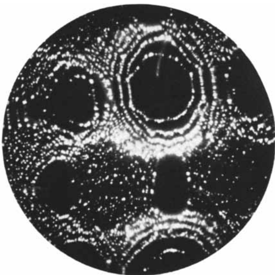
RHENIUM NEEDLE TIP is shown in these field ion microscope pictures. The three pictures show successive stages in the evapora-
