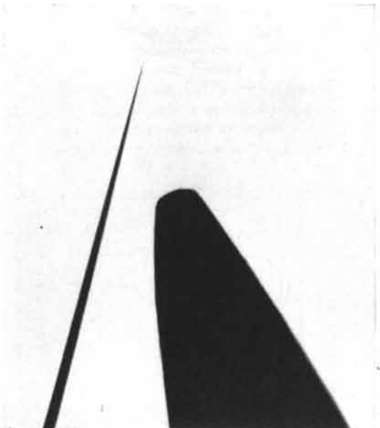
TUNGSTEN NEEDLE of the field emission microscope ( left ) is compared with the tip of an ordinary pin in this photomicrograph.
