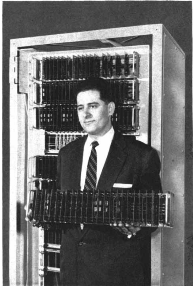
FICo digital engineer Peter Carbone holding digital module, comprised of easily removable transistorized printed circuits. Rack-type digital computer is in background.
