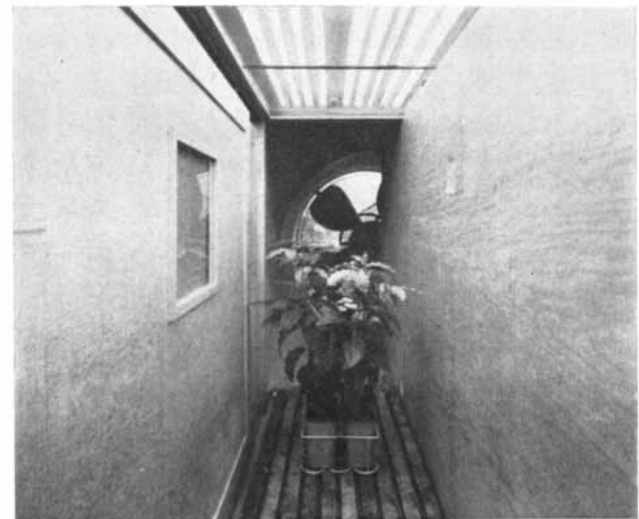
WIND TUNNEL is used to grow plants under various wind conditions. Artificial daylight is provided by the fluorescent lamps at top.
