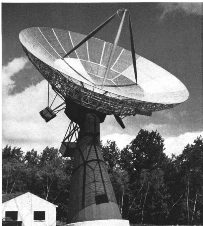
RADIO TELESCOPES which have been used in 21-centimeter absorption studies include the 50-foot instrument at the Naval Research Laboratory in Washington, D.C. (top), and the 60-foot instrument at the Harvard College Observatory's station in Harvard, Mass.
