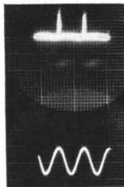
Contact resistance at 140 db sound-pressure level.
