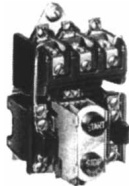
Bulletin 609, 3 Manual Starter. Max. rating: 5 hp, 220 v; 7½ hp, 440-550 v.
