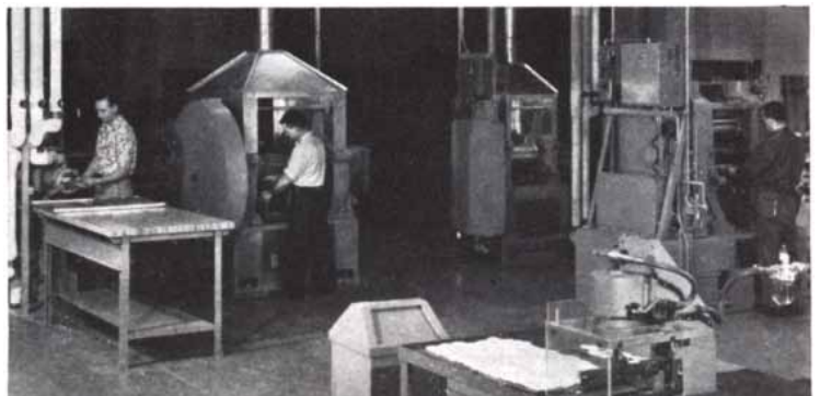
The production process in miniature: The ingredients used to make up each specially formulated compound are carefully blended in the mill (center) to achieve a maximum of homogeneity. The batch is then sheeted out on the calendar (right), or the compound is forced through the extruder. It's then cut into proper lengths for use in the press room, where it is molded according to rigid laboratory specifications.
