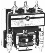
Bulletin 709 Size 4 Automatic Starter—50 hp, 220 v; 100 hp, 440-550 v.
