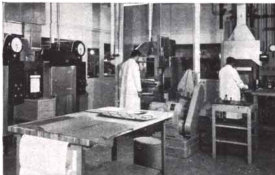
Ovens, mill and press in the Laboratory Section. The entire production of Sirvene parts—from original research to final inspections—is in effect a laboratory process. From the original mixing, through the molding and forming processes and in all final tests, each step is scientifically controlled by Sirvene engineers.
