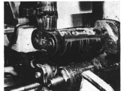
FIG. 3 — Miniature printing press in IBM card machine. Note carbide shearing knives above the printing plate.
