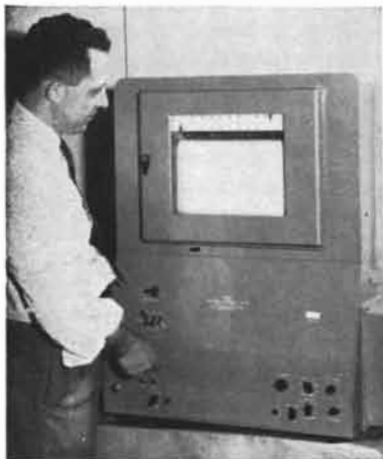
The Cary Model 14 Spectrophotometer provides performance to 1860A, with possibilities for even shorter wavelengths. Heretofore such performance was possible only on custom made instruments.
