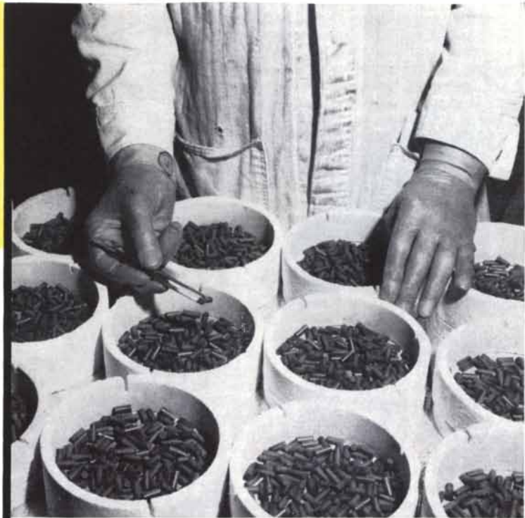
Ceramic Fuel Pellets For Nuclear Reactors. Those illustrated are of a thorium-uranium oxide mixture. They are typical of the ceramic fuel element components available in a wide range of compositions made to exact specifications.
