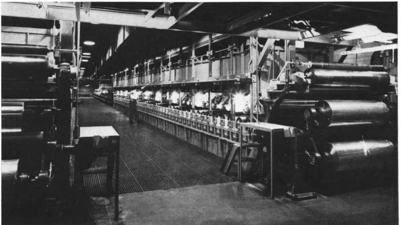
CELLULOSE IS CAST into cellophane in a Richmond, Va., plant of E. I. du Pont de Nemours & Company. Cellulose enters one
