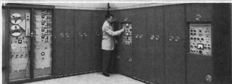
30-channel, analog-digital converter connecting 300-amplifier analog computer to 1103A digital computer
