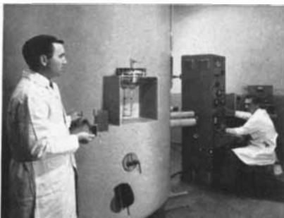
New Laboratory Reactor: Eight-foot-high tank contains fully functional core, coolant and moderator.
