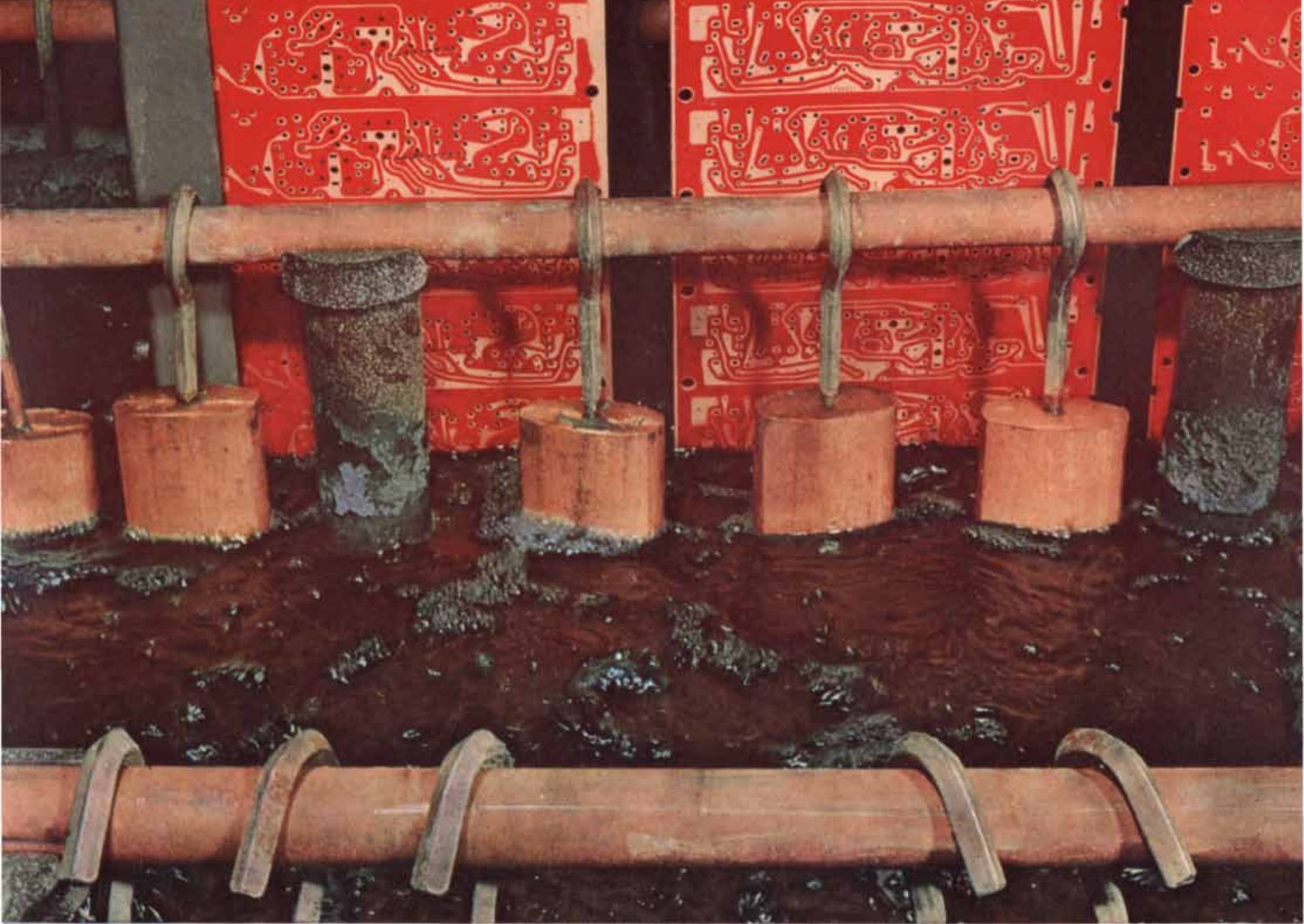
"Plated wiring" for all types of circuits—from radios and TV to auto dashboard panels—is deposited on rows of boards like these in an automatic electroplating tank. Anaconda phosphorized-copper anodes, 42 inches long, hang from the buses.
