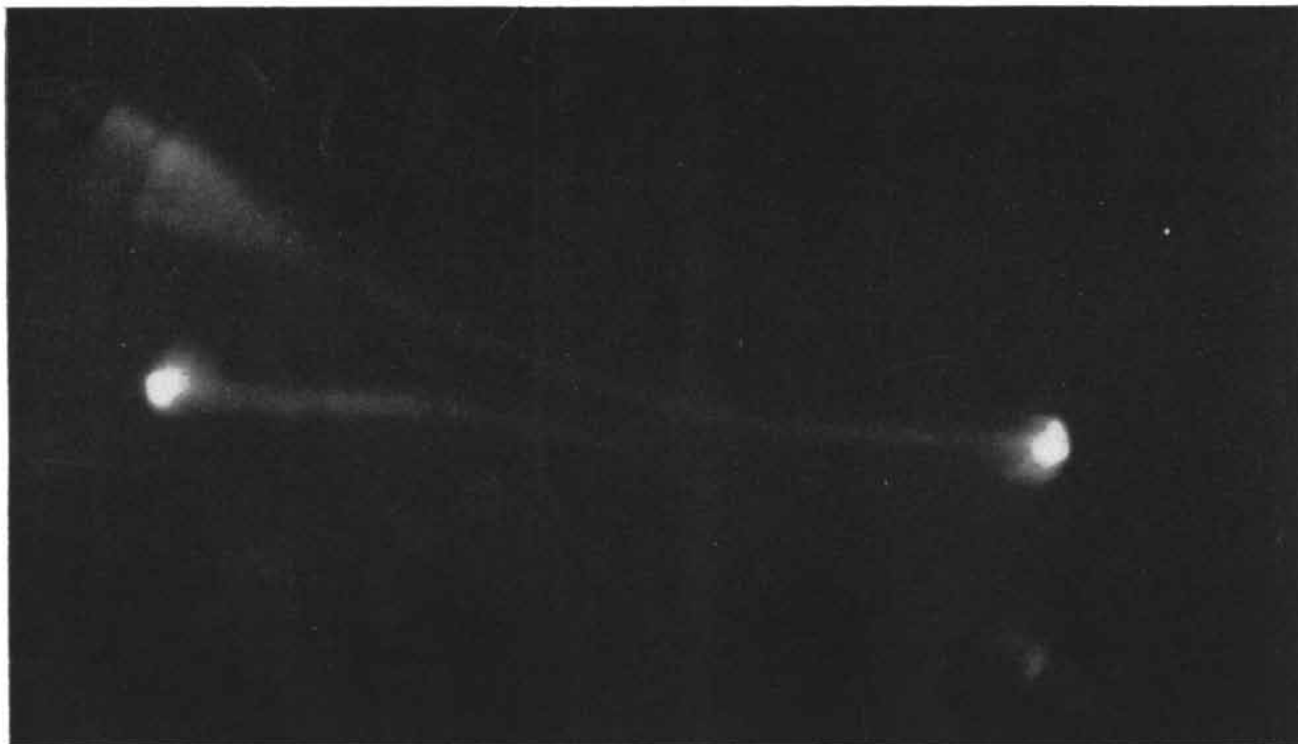
TWO PLASMOIDS are fired at each other in a vacuum chamber containing a strong magnetic field. The initial bursts from the guns are marked by the bright spots at left and right. The lu-
