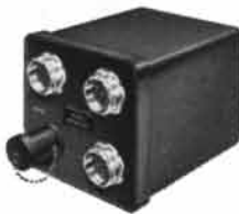
FICo Wind Memory Computer — an aid when navigational systems operate with Doppler.
