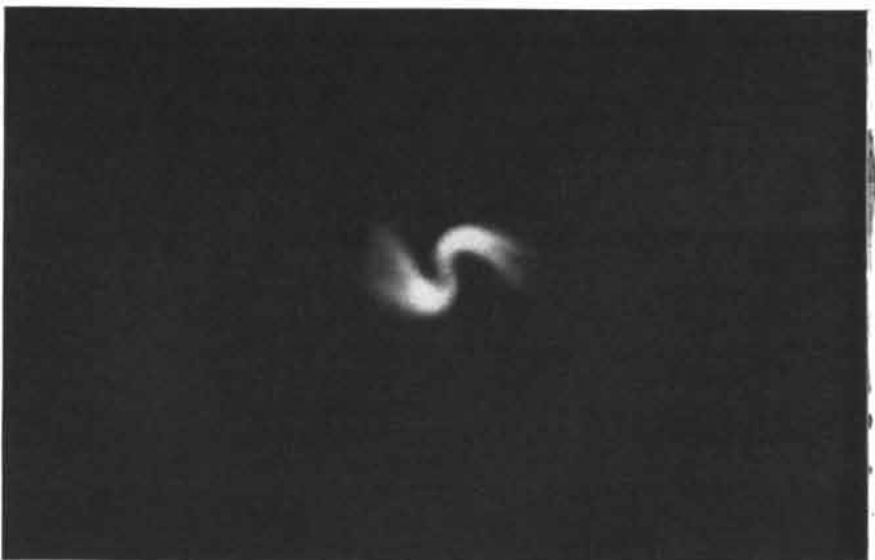
BARRED SPIRAL results when two plasmoids are fired at each other. The photograph at the top of the page is a time exposure; the one at bottom is a two-microsecond "snapshot."
