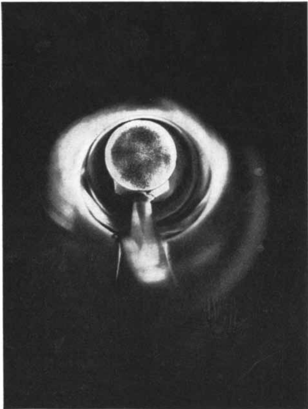
SAMPLE IS LOWERED into apparatus ( left ). Around it is the silvered wall of an insulating Dewar flask. After an electromag-
