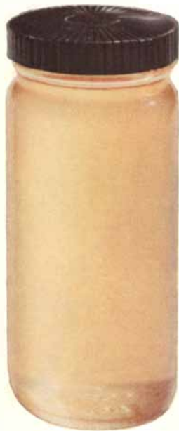
Poor color in this sample of sodium toluene sulfonate resulted from use of competitive nitration-grade toluene.
