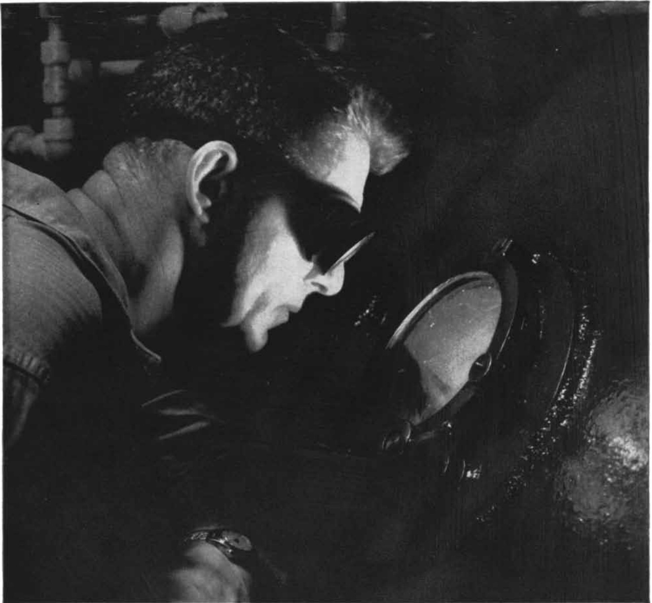
Utica technician viewing a meltdown of Udimet 500—a new vacuum melted alloy in the high temperature field.
