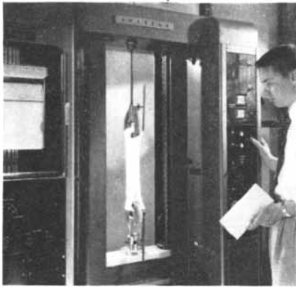
A Chrysler Corporation technician watches as the Instron stretches a piece of foam rubber seat cushioning material to its limit to determine ultimate elongation and tensile strength.
