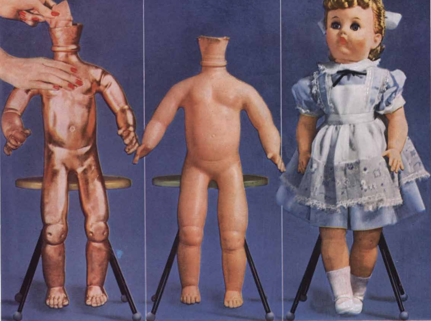
Left: A 9-pound mold of electroformed copper for a 21-inch doll. Soft vinyl "skin" (center) was withdrawn through neck opening. Finished doll at right.
