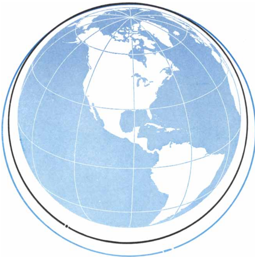
ORBITS OF THE FIRST TWO SATELLITES are shown in relation to the earth, approximately to scale. Orbit of first satellite is in black; of second, in color. The perigee heights are both about 150 miles. The apogees or maximum heights are about 550 and 1,000 miles.
