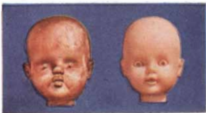
Doll heads also are cast inside molds of electroformed copper — like that shown at left above.
