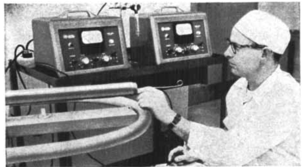
Geiger Counter is used to determine that no radioisotopes have penetrated into the interior of the repeater unit.
