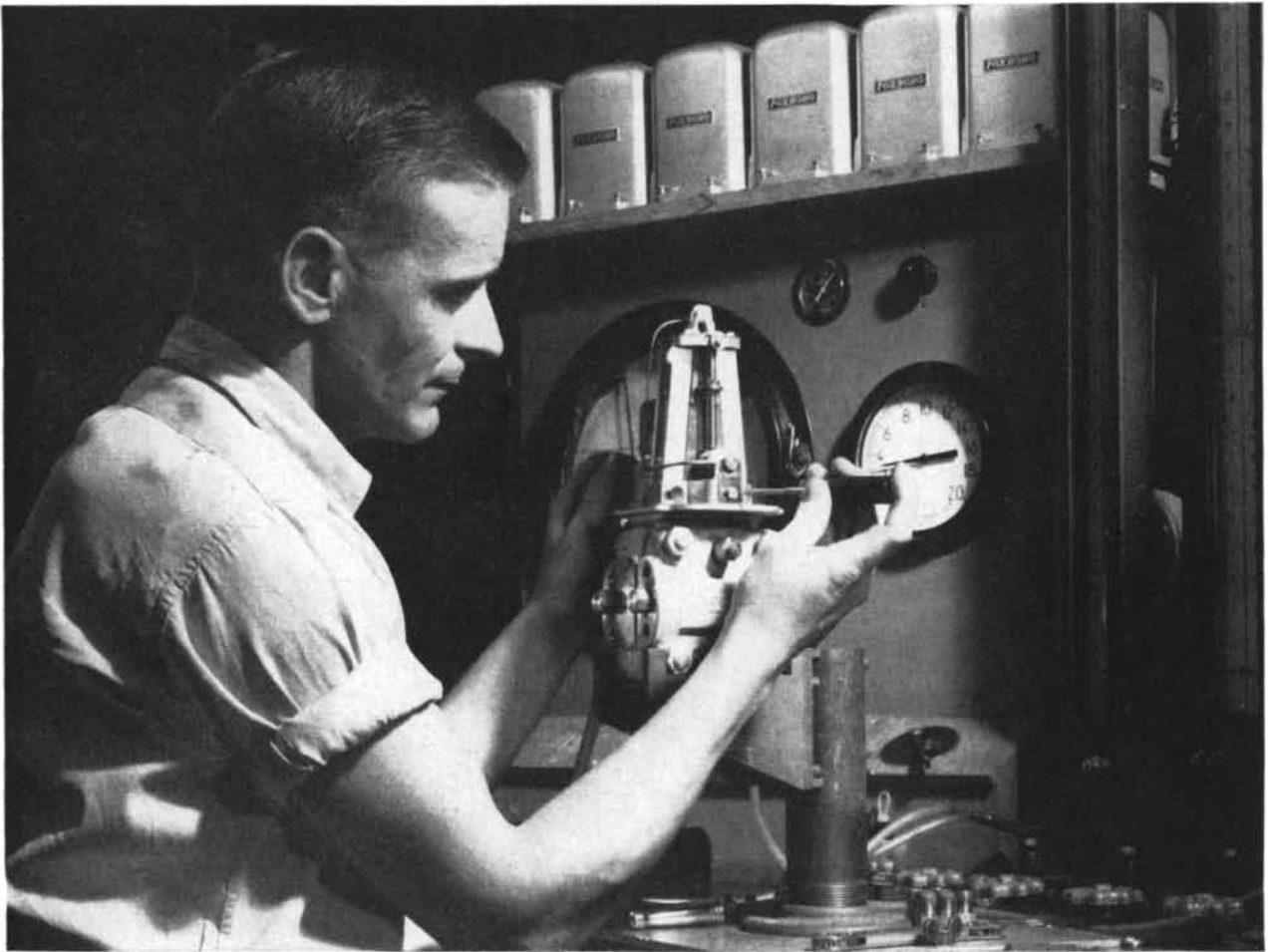
Precision calibration of the d/p Cell Flow Transmitter — a Foxboro development which has improved processing accuracy in more than 60,000 installations.
