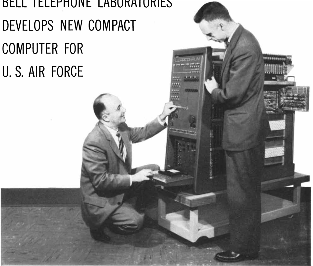
J. A. Githens, B.S. in E.E., Drexel Institute of Technology, and J. A. Baird, Ph.D. in E.E., Texas A. & M., check the control panel of Leprechaun, a new high-speed computer which solves extremely complex problems in one-tenth of a second. Small size and low power are made possible by new design principles and Bell Laboratories' invention of the transistor.
