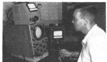
Engineer at Ford Instrument tests jet engine exhaust temperature indicator developed for the Navy's Bureau of Aeronautics.
