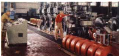
Modern high-speed rolling mill specially installed by The American Brass Company to produce radiator copper.
