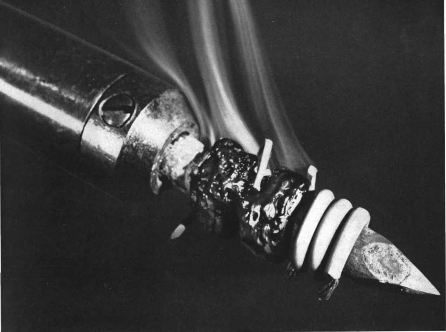
It's easy to tell which are the TEFLON TFE-fluorocarbon resins . . . as other wire insulations (Fig. A) soften, (Fig. B) melt, and (above) finally char.
