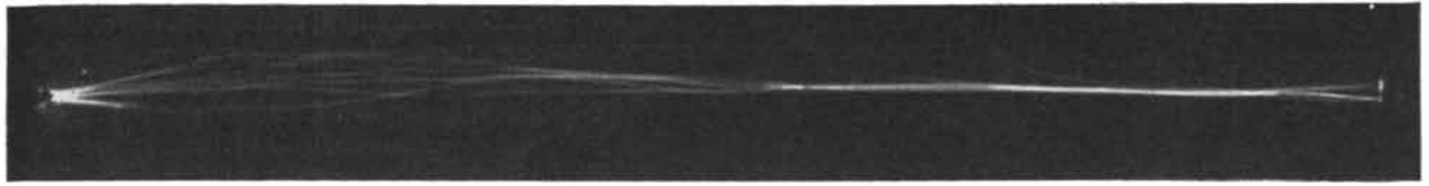
Erratic spark discharge at a pressure of 1.5 centimeters of mercury
