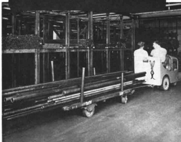
Compressed blocks of Wellington Sears duck are used in Divine Bros. Canvas Cushion Tired Wheels on this factory truck.
