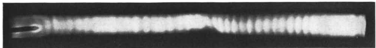
Disks are distorted (center) by the application of a magnetic field
