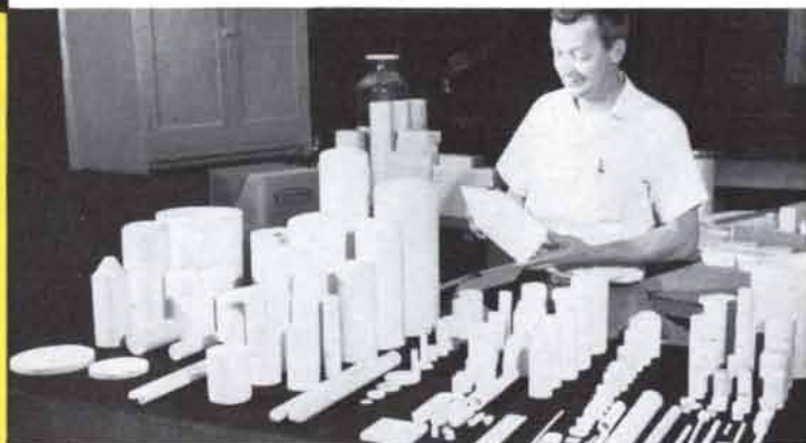
High Purity Refractories Vital To Metallurgy include crucibles, made of MAGNORITE* pure magnesia, zirconia and thoria, suitable for melting uranium, plutonium, thorium, etc. A special Norton laboratory devoted exclusively to nuclear problems is developing other unique ceramics for the atomic program.
