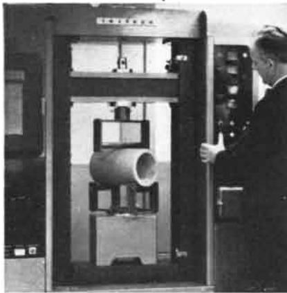
At the Owens-Corning Fiberglas Product Testing Laboratories, the Instron performs a strength test on Fiberglas Prefabricated Duct (a highly efficient air-conditioning air transfer product) to compare its crushing strength with that of old-type metal ducts.
