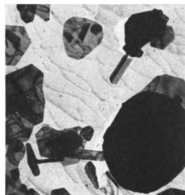
Undissolved silicon (large opaque particles) and thin silicon plates in an aluminum matrix, magnification 12,000 diameters. (Micrograph courtesy General Motors Research Staff.)
