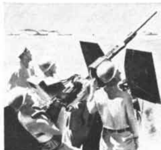
1942 Ship defense against aircraft was greatly strengthened by introduction of Sperry's gyroscopic computing gunsight.
