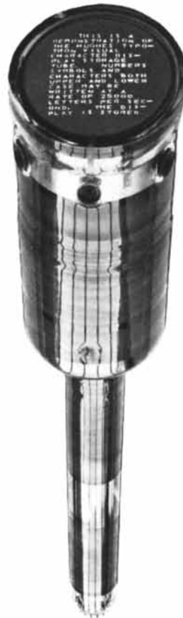
The TYPOTRON tube displays information in the form of letters and symbols.
