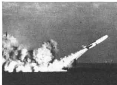
1953 Navy's Regulus missile, built by Chance-Vought for ship or submarine launching, is directed over great distance to target by Sperry gyroscopic controls.
