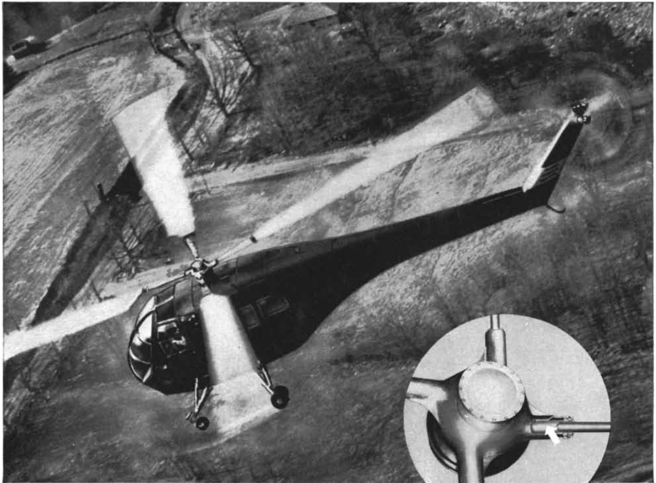
SLEEVE BEARING of Du Pont ZYTEL used in rotor hub of helicopter eliminates field maintenance of blade-retention system. (Made by Doman Helicopters, Inc., Danbury, Conn.)
