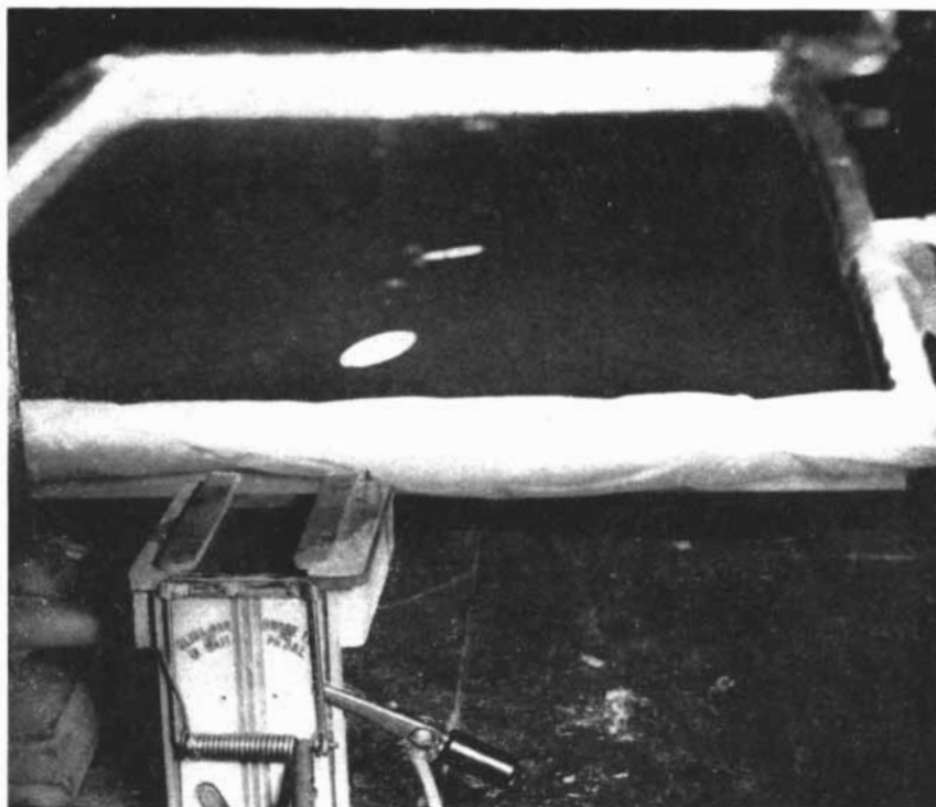
Van Riper's apparatus for making high-speed photographs of a skipping button
