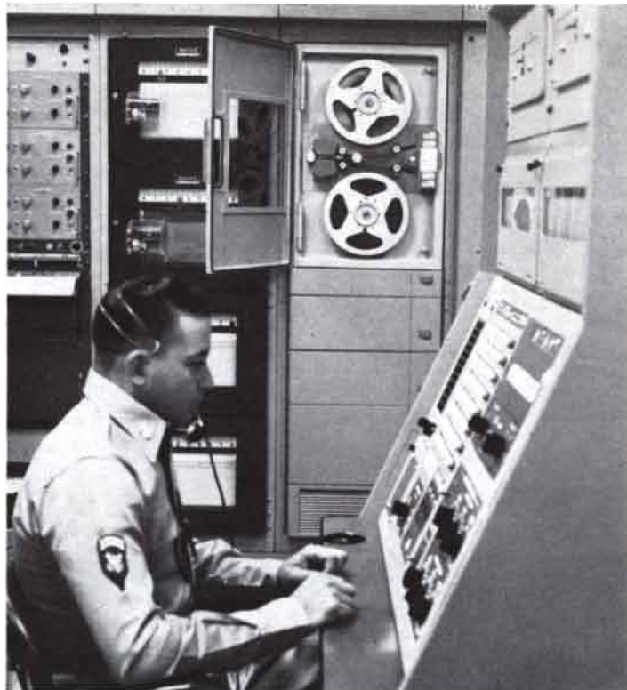
Simulation control console showing the Ampex FR-100 behind
