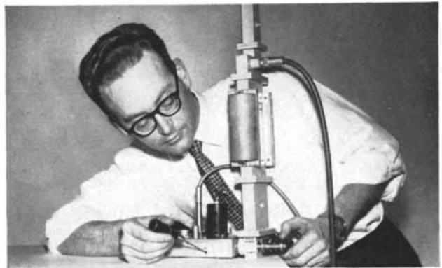
Peter Sandsmark, from Polytechnic Institute of Brooklyn, and his fellow electrical engineers develop a new microwave radio relay system able to transmit three times as much information as any existing system. Objective: more and better coast-to-coast transmission for telephone conversations and network television.
