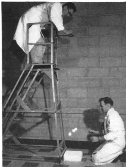
Egg bouncing from 12-foot drop demonstrates superior cushioning properties of flexible urethane foam.
