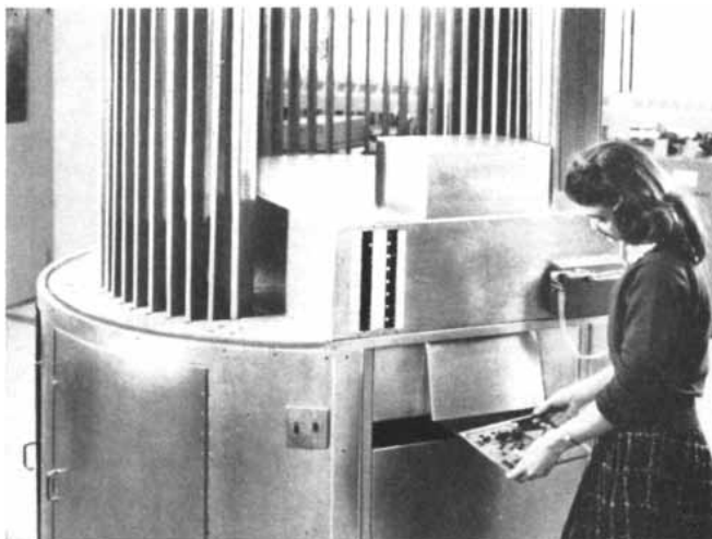
This 7-foot high machine can handle up to 50 different components stored in the magazines on top. These components are mechanically selected and mounted on carrier circuit boards by use of a punched
