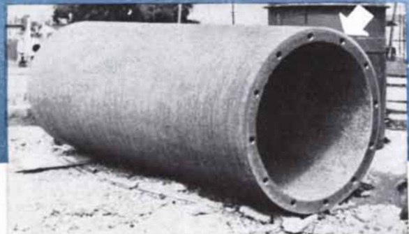
54" o.d. section of finished pile showing precise round channels formed by U. S. Rubber Tubing. There are 12 of these cores in every section. Each core has a diameter of 1.375 inches.
