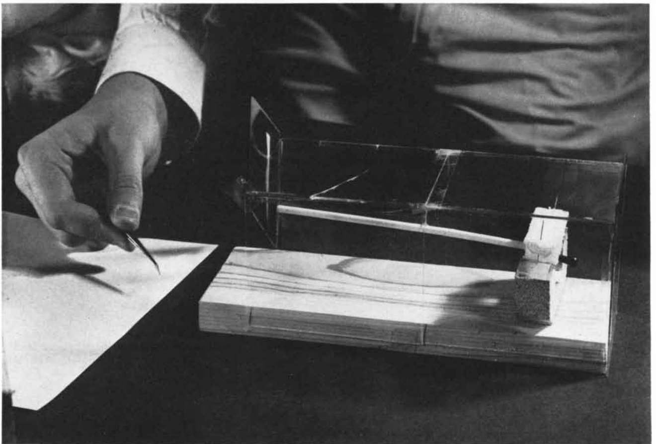
MICROBALANCE is made of a drinking straw, wood screw and other simple materials. The arm balances on a pair of needles resting on a glass slide. At top left a student places a standard
