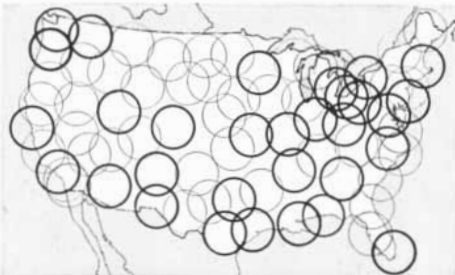
Raytheon radars at 27 of the 31 heavily circled areas will soon be operating as part of C.A.A.'s flight control network. Light circles indicate future coverage.
