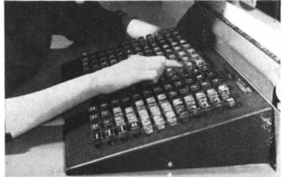
Working from a standard planning sheet a typist (with only one hour of training) can punch a HUGHES digital control tape on the self-correcting keyboard.
