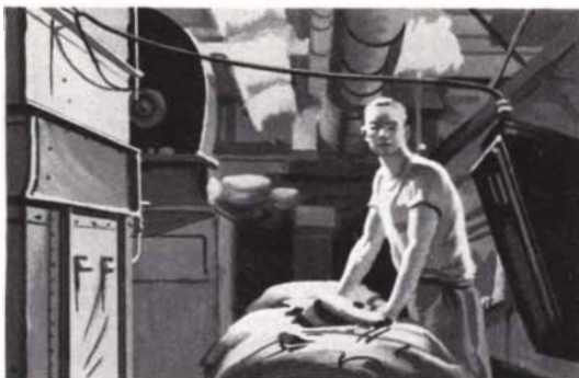
Special grease saves $1,075. Six blower breakdowns a year were occurring in ovens used to dry leather. 300°F. temperatures caused bearings to fail. Mobil recommended high temperature grease. Failures ceased, grease consumption was cut 50%.
