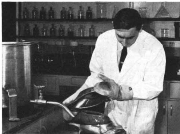
A new concept of plastics manufacture—slush molding with A-C polyethylene. (Decoys at left are from mold above.)
