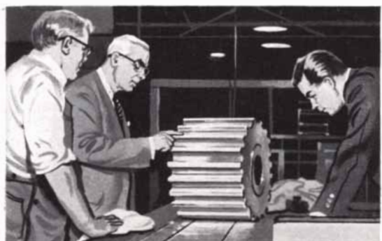
Mobil specialist avoids costly gear replacement. Mobil gear specialist made a study of all gears in Endicott Johnson's Paracord plant. His recommendation to reverse certain gears to compensate for wear avoided replacement... saved a substantial sum.
