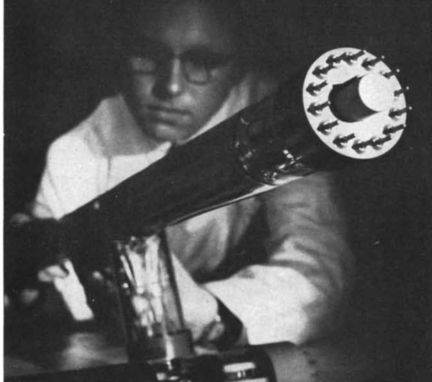
Laboratory research often occupies a considerable amount of the scientist's time. Here a scientist examines an experimental tube for testing photosensitive devices.
