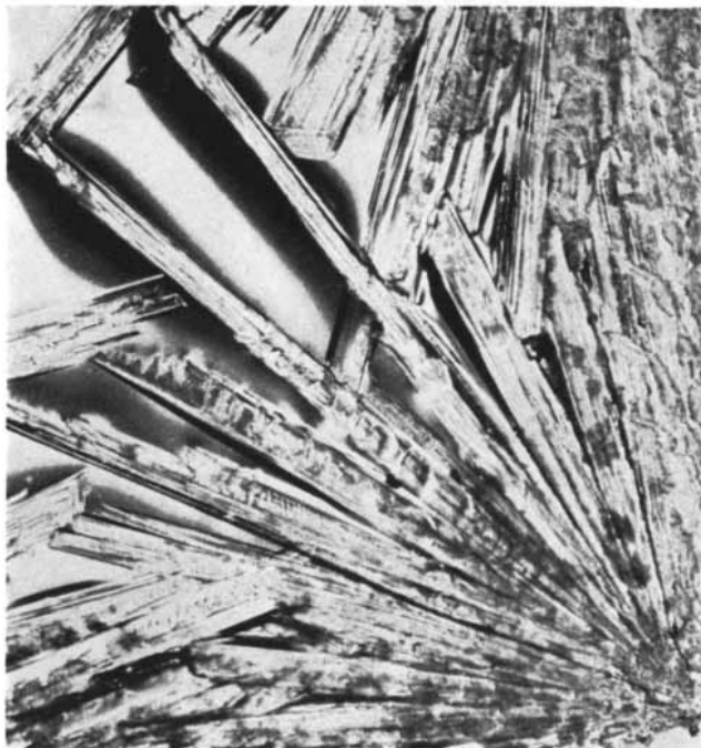
3 Crystals have now engulfed 75% of area. When determined, the freezing point is compared with that of 100 mole % phthalic anhydride—permitting accurate calculation of over-all purity.
