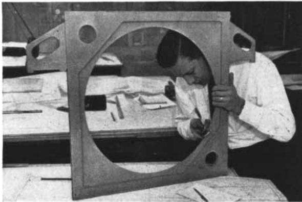
Casting of thin-walled close-dimensioned parts. Tennessee Eastman filter frame plate previously required a good deal of careful milling on thin inner web. Combined use of shell core in a sand mold held tolerances, eliminated milling operation.
