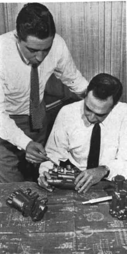
Casting of intricate parts: Jet engine afterburner component, cast for Pratt & Whitney Aircraft by Cooper Alloy, is a tangle of projections and cavities. Required, however, were the most precise dimensions to make for automatic precision machining. Shellcast® shell coring and CO 2 process cut down rejection and machining costs.
