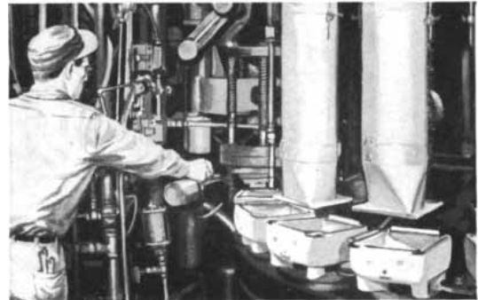
Shear spray lubricant saves $11,175 —In automatic glass-forming machines, steel shears that cut molten glass were pitting, rusting, leaving excessive "shear" marks on molded material. Mobil introduced product, about 1/10 cost of previous lubricant, to cut reject rate, reduce maintenance and parts replacement.
