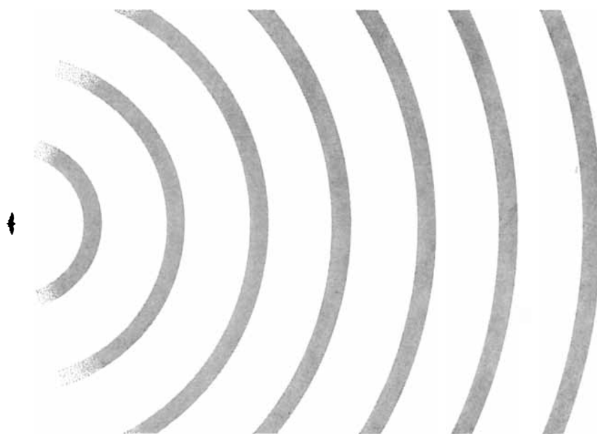
WIDE BEAM of short, frequency-modulated pulses is emitted by most bats while hunting. Each pulse (gray curves) is about 1.5 feet long. Beam is fixed with respect to bat's head.
