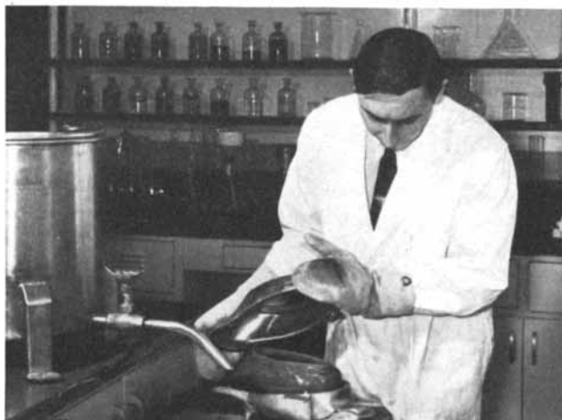
A new concept of plastics manufacture—slush molding with A-C polyethylene. (Decoys shown are from mold above.)
