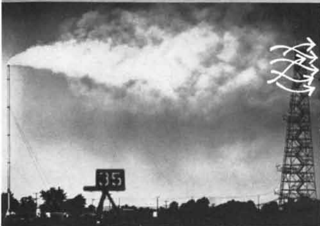
Multiple exposure photograph of a smoke plume from the Meteorology experimental stack.
