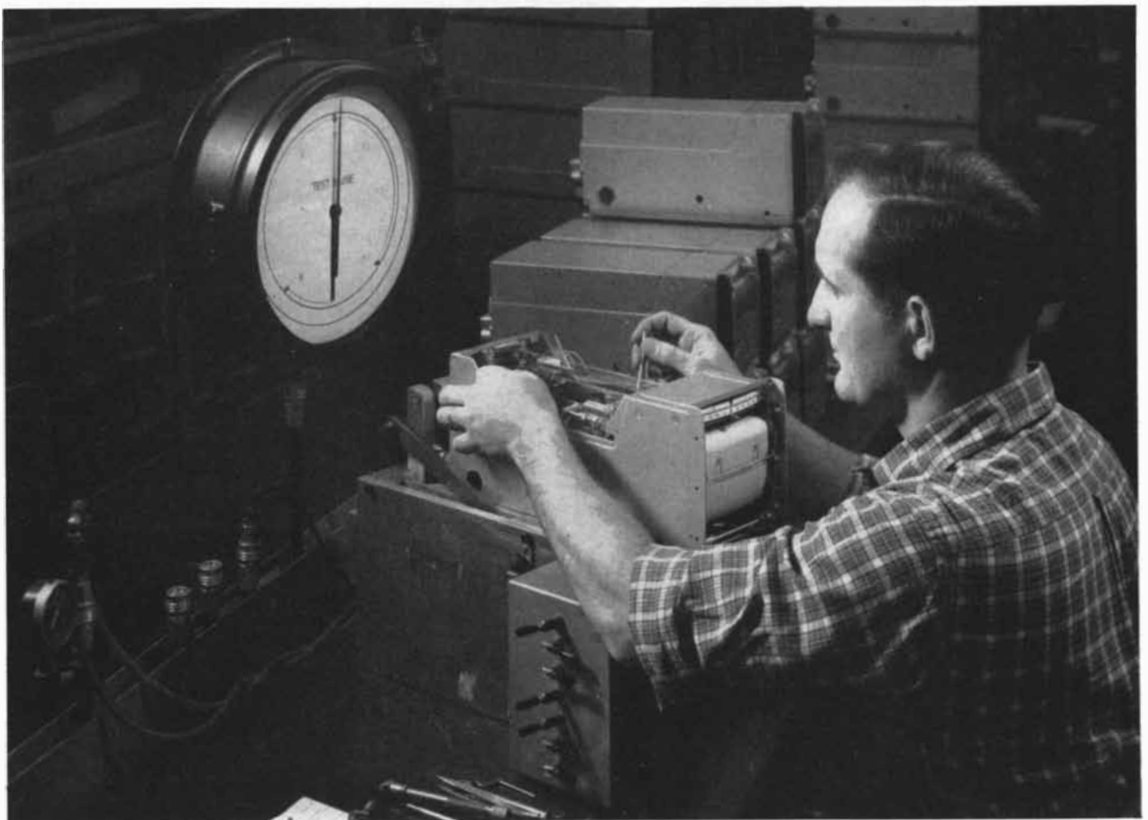
Consotrol Control Station undergoing final calibration. Full 4-inch chart width is one of many advances in small-case panel instruments introduced by this Foxboro development.
