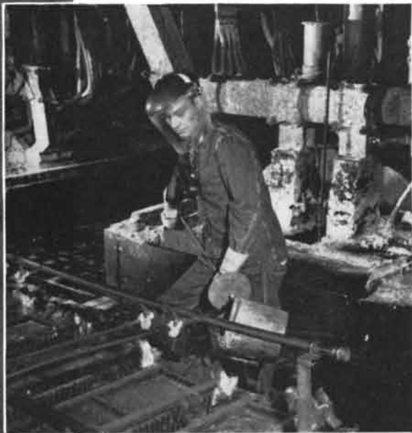
METAL FROM THE SEA: Molten magnesium, 99.9% pure, is shown above being ladled into molds at the Texas Division of The Dow Chemical Company. Electrolytic cell in background, which separates the metal from magnesium chloride, must withstand intensely corrosive action of liberated chlorine gas. Blocks of MONOFRAX® a material by Carborundum with high resistance to heat and corrosion, solve the problem.
