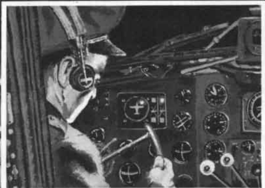
Aircraft Proximity Warning System utilizes modulated beams of light to detect the approach of aircraft from any direction as far away as 5 to 7 miles.
