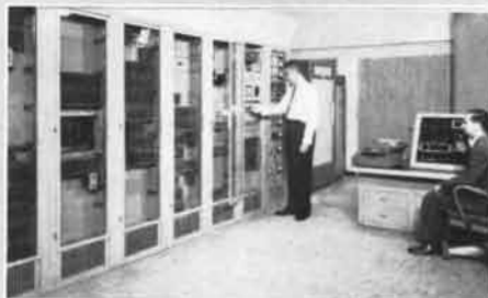
Data conversion system for digitizing and processing telemetered missile test data.
