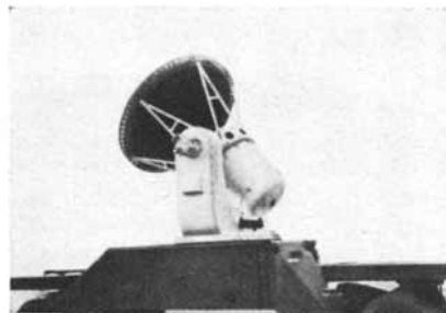
NIKE GROUND GUIDANCE—Large magnesium assemblies are easily and effectively protected by standard finishing methods.
