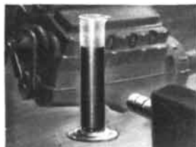
Checking durability of pistons—radioactively treated—by measuring radioactivity of worn particles deposited in the oil
