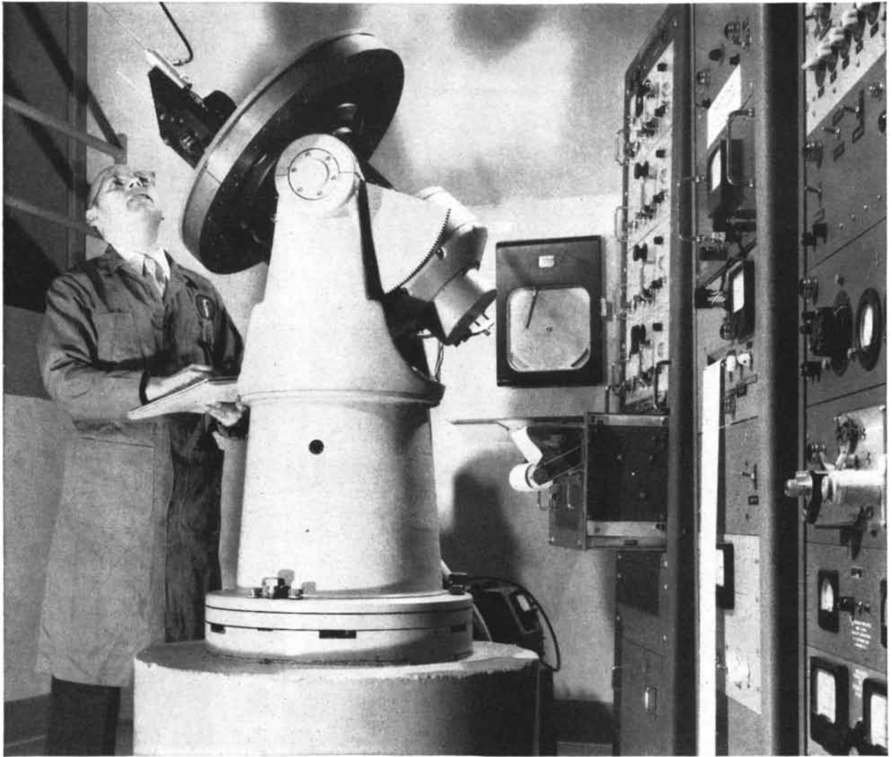
Ford Instrument Co. Engineer checks air-bearing gyro for angular drift on equatorial test stand. Test can show up drift rates as low as one revolution in 40 years. Tests like this . . .
