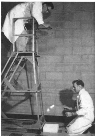
Egg bouncing from 12-foot drop demonstrates superior cushioning properties of flexible urethane foam.
