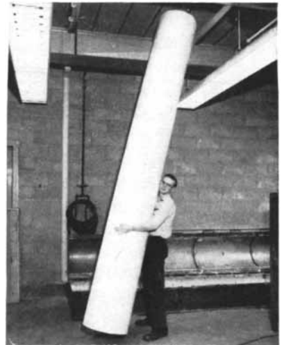
Buoy for dock has rigid urethane foam core, polyester-glass fiber surface—resists shock, marine growth.
