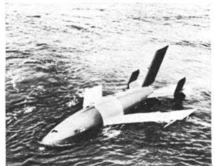
RYAN FIREBEE, with 75% of its exterior surface magnesium, has withstood repeated dunkings in the ocean with no adverse effects. The reason—Ryan applied the proper protective measures.
