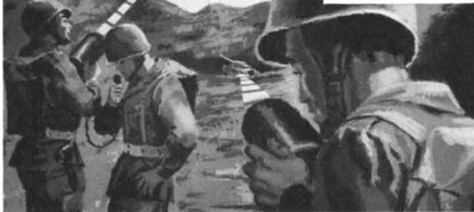
Interception-proof Military Communication System employs invisible, jam-proof light to transmit vital voice messages in air-to-air, air-to-ground, and ground-to-ground communications.
