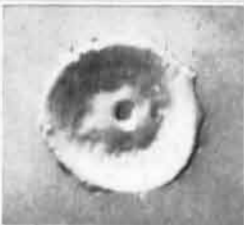
Electron micrograph of impact produced on aluminum coated glass by a 1 micron diameter particle traveling at 7,000 feet per second.
